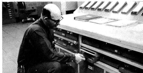
Fig. 4. The radio control console providing city wide communications and communications directed to the individual boroughs.
