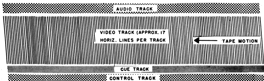
FIG. 2a TRANSVERSE TRACK (2 IN TAPE, QUADRATURE HEAD)
