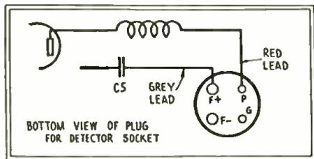
Detail of the plug used to connect the adapter-receiver to the amplifier of a broadcast set, by Fahnestock clips to C5 and the plate choke LA.
