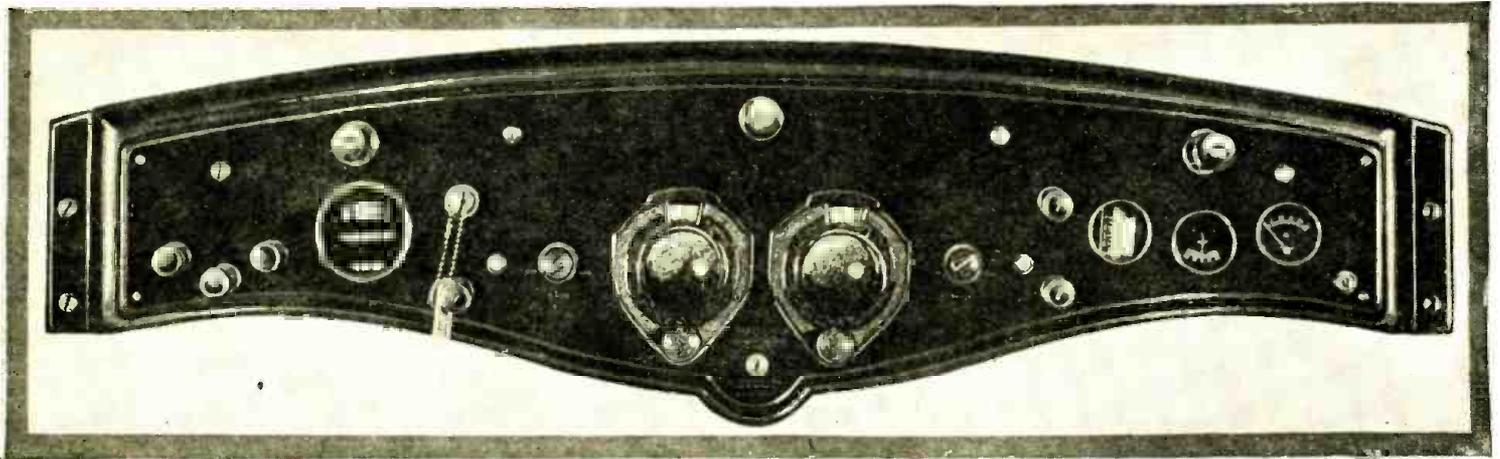
The radio-equipped automobile has a special instrument board, including the radio controls, which replaces the old panel.
