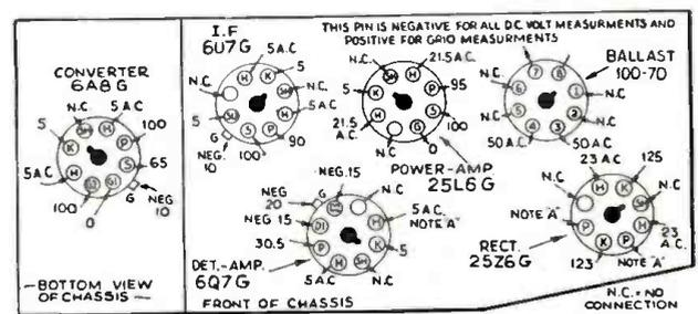
Voltages measured from No. 7 pin on ballast tube to point indicated using a 1,000 ohms/volt meter. Vol. control at minimum. Antenna disconnected. All filament voltages measured across each respective tube, using a 0-30-V. A.C. voltmeter.
