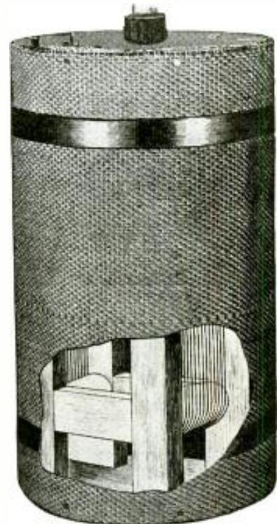
A shield around the loop stops static.
