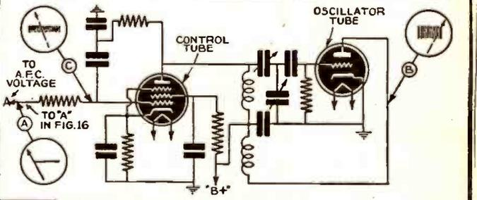
FIG. 17 ~TYPICAL CONTROL CIRCUIT FOR A.F.C.~
