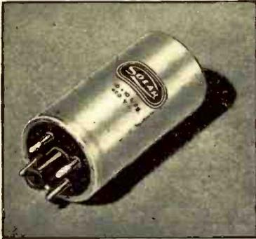
**A** NEW series of dry electrolytic condensers in metal cans which may be plugged into a socket as easily as a radio tube. Known as Type DO, they can be easily removed for both testing and replacing. To insure rigidity of mounting for marine and aviation service, straps are available for holding the condensers in their sockets.—*Radio-Craft*
