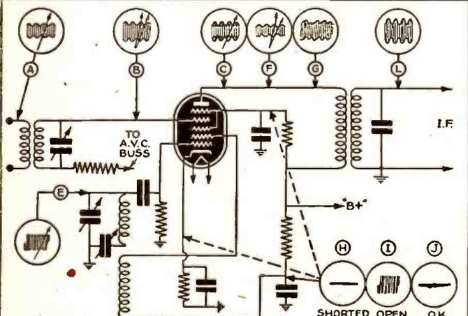
FIG. 12 ~TYPICAL 1ST-DETECTOR & OSCILLATOR USING MULTIPURPOSE TUBE.~
