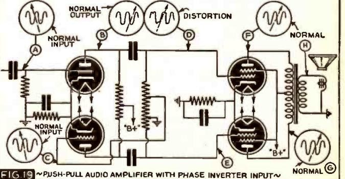
FIG. 19 ~PUSH-PULL AUDIO AMPLIFIER WITH PHASE INVERTER INPUT~
