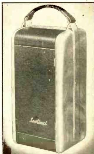
Sentinel camera-type portable receiver. Overall cabinet dimensions, 4 7/16 x 4 x 8 13/16 ins.; weight, complete with batteries, 4½ lbs. Since the loop antenna is built into the receiver, it is necessary to rotate entire set for maximum signal pick-up.
