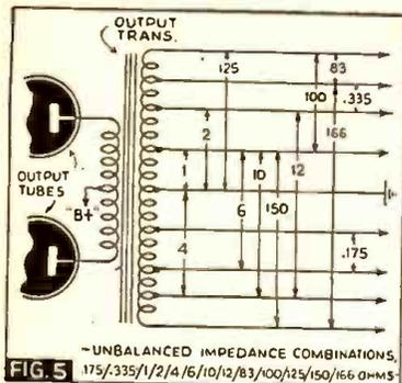
FIG. 5 - UNBALANCED IMPEDANCE COMBINATIONS, 175/.335/1/2/4/6/10/12/83/100/125/150/166 OHMS
