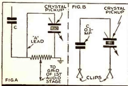
● TO SAVE time when adding phonograph pickups to radio receivers, place the pickup across the volume control, as shown at A in the illustration above.
