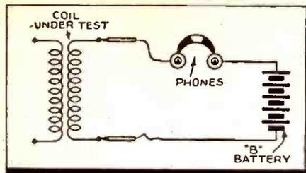
● I HAVE found earphones connected in series with a "B" battery and a pair of test leads, as shown in the diagram, to be the best method of locating noisy R.F., oscillator and I.F. coils. The radio set under test is disconnected from the power supply and a test is made across each winding of each coil, and also from the primary to the secondary winding. The same method may be used in locating noisy resistors and condensers.
