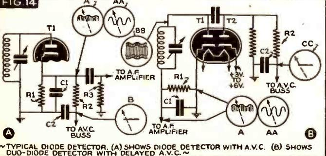
FIG. 14 ~TYPICAL DIODE DETECTOR. (A) SHOWS DIODE DETECTOR WITH A.V.C. (B) SHOWS DUO-DIODE DETECTOR WITH DELAYED A.V.C.~
