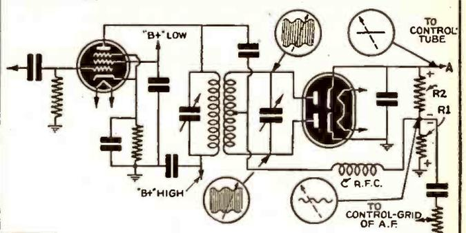
FIG. 16 ~TYPICAL FREQUENCY DISCRIMINATOR CIRCUIT FOR A.F.C.~
