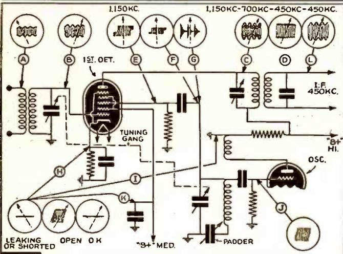
FIG. 11 ~TYPICAL 1ST-DETECTOR & OSCILLATOR USING SEPARATE TUBES.~
