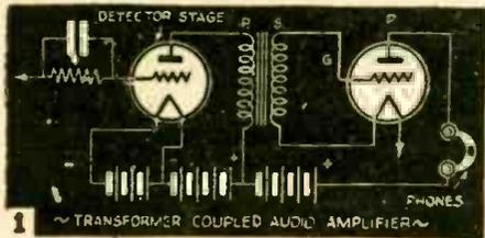
receivers it consists of only one stage, the power stage (also called output stage). In older receivers, and in some special high-fidelity models, there were two or more stages following the detector, called "First A.F." stage, "Second A.F." stage, etc.
