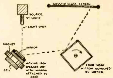
a screen, small hole and lens) is focused on to a small mirror attached to armature of an old magnetic type loudspeaker unit.
