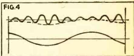
Fig. 4—The modulated beat frequency after detection a second time, leaving the audio frequency component.
