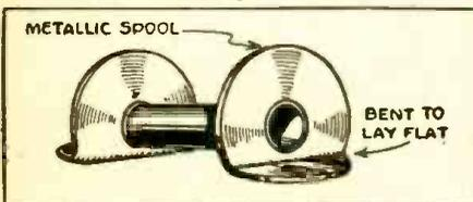
Just simply bend the ends of the spool as shown in the sketch so that it lies flat on the table and supports the iron, and keeps it from sliding or rolling.
