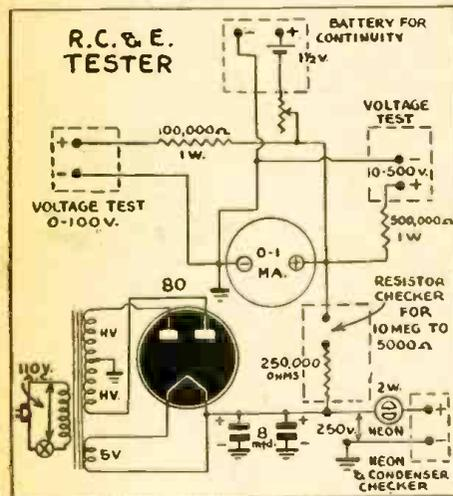
be calibrated in this way. Get several good resistors and find out their reading on the meter and fill in the rest by mathematics. My power transformer was 2 1/2 by 4 inches. The neon bulb is of the 2-watt type as all others will burn out.
