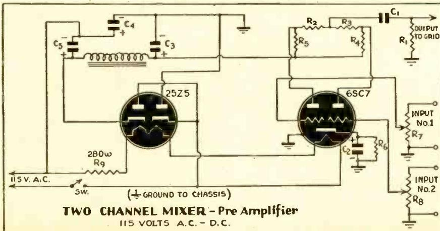
This diagram shows a self-powered, high gain, two-channel mixer pre-amplifier. It uses a 25Z5 and a 6SC7 in an A.C.-D.C. circuit.
