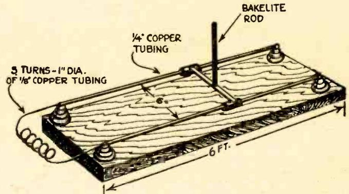
holding the rod to the copper shorting bar. The system should be kept in the clear and as far distant from surrounding stray fields and metal as is practicable under ordinary circumstances. The distances between nodes will represent half a wavelength.
