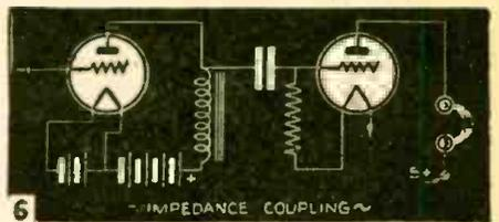
rent (necessary to maintain the plate at a positive potential) may cause distortion. This is especially true in audio transformers having a very small iron core, such that the direct current causes it to become *saturated* by the magnetic field. The use of a larger core will reduce the amount of distortion, but may cause certain losses.
