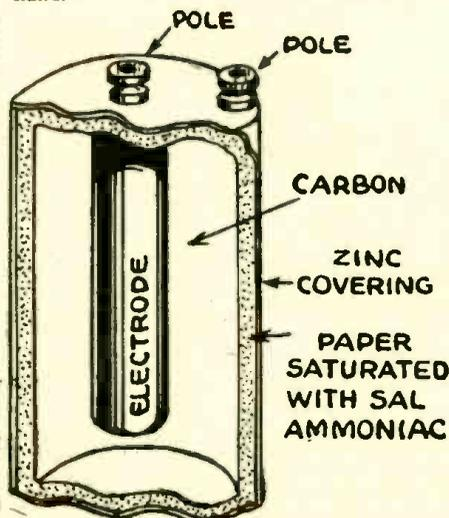
All you have to do is to secure one or two 1½ volt dry cells, large size (see drawing).
