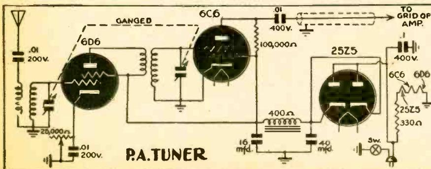
**SOMETIMES** a simple R.F. tuner is needed to bring in just a few of the powerful local stations, to be operated through a small public address system. Almost anything will do, as a rule.
