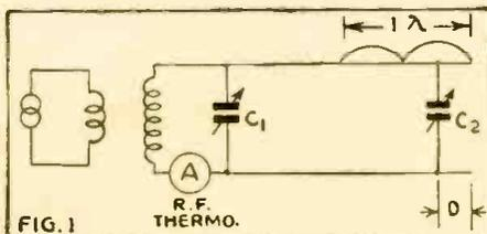
made equal to the reactance of the cut-out section, the surge impedance is equal to  $Z_0$ , and is found by varying the setting of C2 until the circuit is again resonant.
