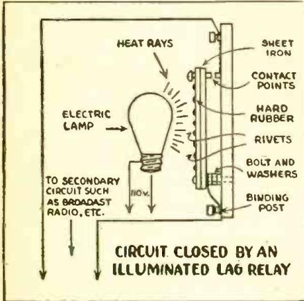
When the lamp is turned on it will be a matter of seconds before the heat from the lamp causes the strip of sheet iron to bend from its expansion. This causes the two contact points to touch and thus complete the secondary circuit. Its application is shown in the diagrams.—L. B. ROBBINS
