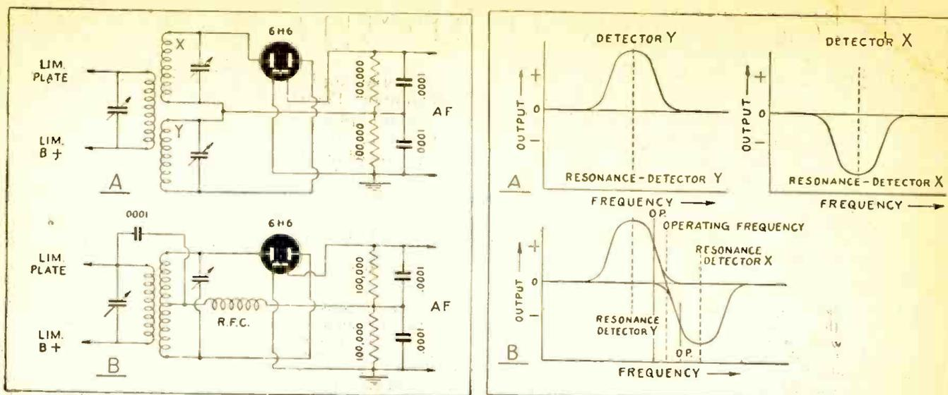
Fig. 1, left—Two fundamental FM discriminator circuits. The system at B is the one now commonly used in commercial FM receivers. Fig. 2, right—How the two separate AM detectors of Fig. 1-A can be made to operate as a discriminator for detecting FM signals.
