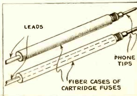
The leads were attached to the phone tips, threaded through the case, and the tips were forced into place as in the diagram.
