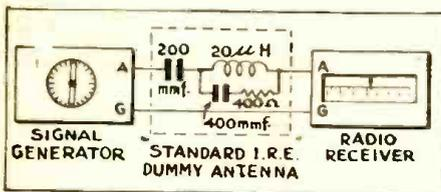
Fig. 1—A receiver is used for calibration.
