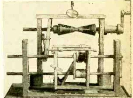
securely in the cone, then face the collar of each piece of spool with tin so as to give smooth bearing and prevent undue friction and wear. A piece of metal should also be placed inside one winding post.
