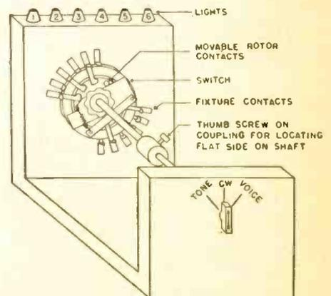
FIXTURE FOR TESTING SIGNAL SELECTOR SWITCH
