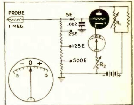
Fig. 2—The vacuum-tube voltmeter described.
