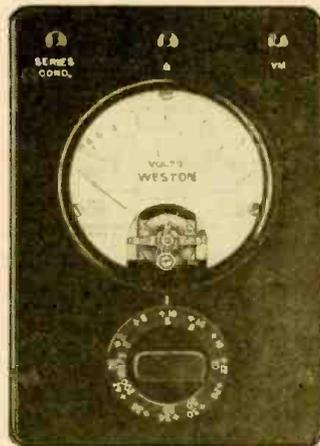
provides readings in decibels as well as in volts. Thus it is ideal for power level measurements in all types of sound equipment and in radio receivers—as well as A.C. voltage measurements from 2 to 200 volts full scale.
