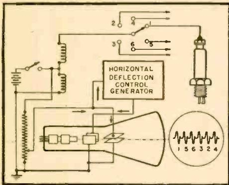
A voltage divider across the primary picks off a suitable voltage. This is applied to both sets of deflecting plates of the oscilloscope. In addition, the horizontal plates are influenced by a deflection control generator connected in series. The frequency of the latter is adjusted to the  $n$ th sub-multiple of the breaker point frequency, where  $n$  is the number of cylinders in the particular engine.
