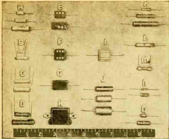
A-D are ceramic, E-H mica, and I, J, ceramic capacitors. K to O, are carbon resistors.
