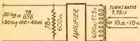
Fig. 2—Gain calculations for an amplifier.
