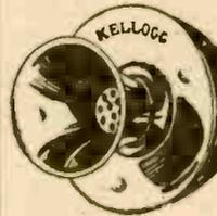
These are regular "telephone transmitters" of the type used on wall telephones. Taken from a junkyard telephone supply company's overstock, these also make offer a grand opportunity to obtain a splendid unit for little more than the price usually asked for a simple microphone button.
