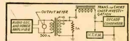
Fig. 3—A Comparator for audio frequencies.
