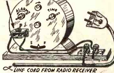
Merely set the clock to ring at the end of your favorite program. When it goes off, the wing nut turns the switch to "off" automatically.
