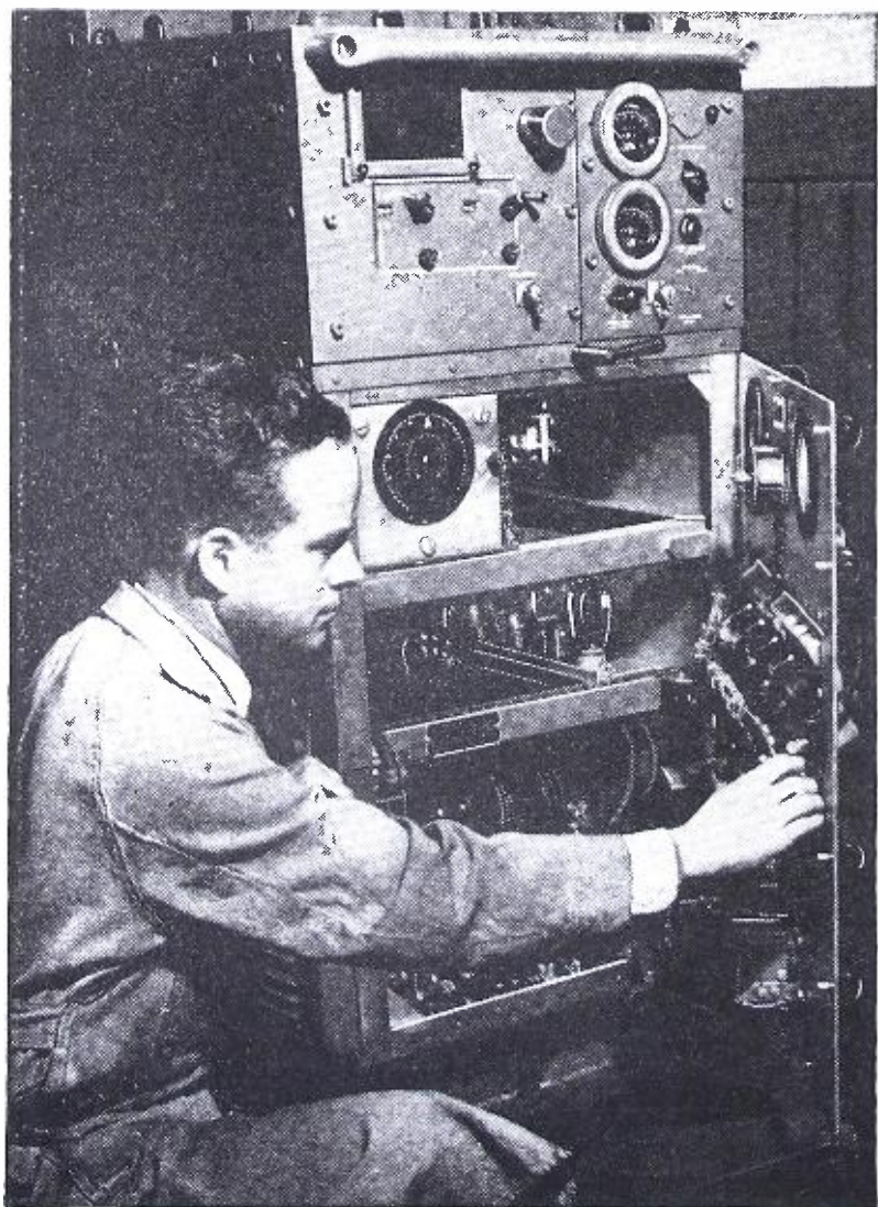
A—Ultra-high-frequency anti-radar transmitter partly open to view. B—Direction finder, center, in an array of anti-radar apparatus.
