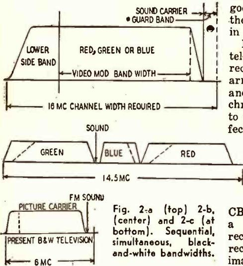
Fig. 2-a (top) 2-b. (center) and 2-c (at bottom). Sequential, simultaneous, black-and-white bandwidths.
