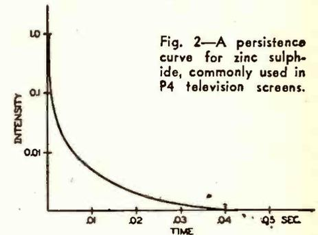
Fig. 2—A persistence curve for zinc sulphide, commonly used in P4 television screens.
