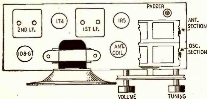
This layout, with slight modifications, can be used with any parts.
