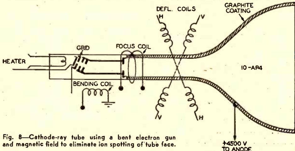
Fig. 8—Cathode-ray tube using a bent electron gun and magnetic field to eliminate ion spotting of tube face.
