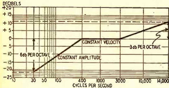
Fig. 4—The recording characteristic curve for frr recordings.
