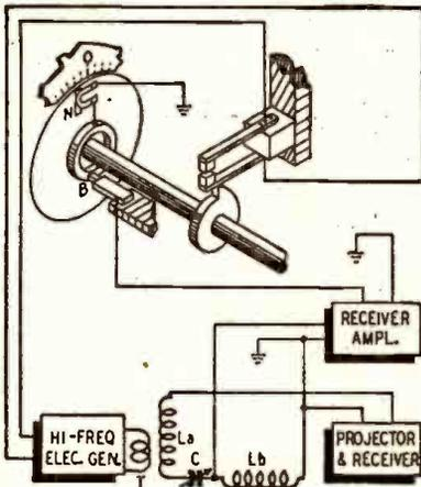
instant that the slot corresponds to zero on the scale. Received pulse echoes are applied across the neon tube which is caused to glow during such instants. Since transmission of a pulse takes place while the slot is at zero, the echo will arrive after the slot has moved to some other position. If the scale calibration is marked off in suitable units of distance, the range of an object is indicated directly by noting the point at which the neon tube flashes.
