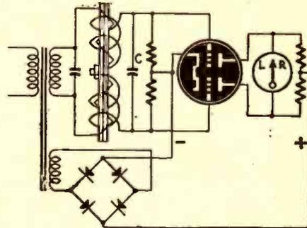
space, it may be considered as composed of two equal and opposing electromagnets, end to end. Since hysteresis lag depends upon peak magnetism, it is equal for each half of the core in this case and there can be no induced secondary voltage.
