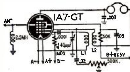
1A7-GT with the detector coils connected between the No. 1 and No. 2 grids. This permits the plate to operate at full voltage without the coupling resistor normally used for interstage coupling to an a.f. amplifier. The plate is coupled to the detector by the electron stream. Regeneration is controlled with a 0.02- $\mu$ f condenser in series between the No. 2 grid and ground.
