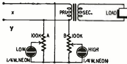
Two 100,000-ohm wire-wound potentiometers are connected in parallel across the a.c. line. The lamps are connected between the arm and one end of the potentiometer. If it is desirable to establish limits between 100 and 120 volts (for example), the potentiometer A is adjusted so that its neon lamp starts to glow when 100 volts is applied across X and Y. Potentiometer B is adjusted so that its lamp glows with 120 volts on X and Y. An autotransformer is useful in making these adjustments.
