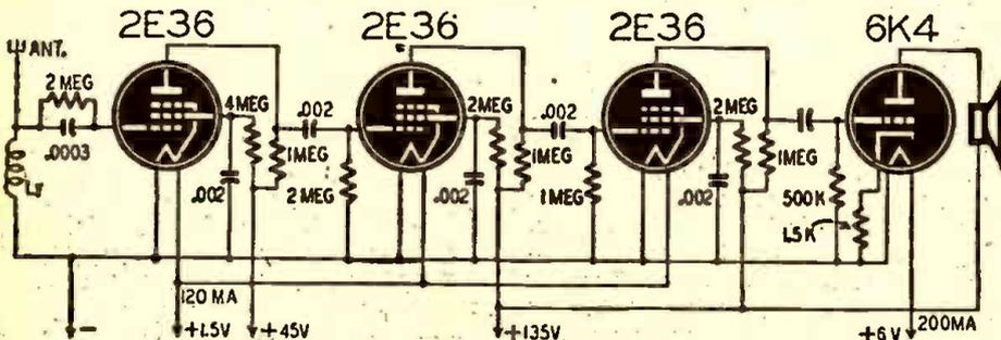
Fig. 3—Hookup of the 4-tube printed receiver does not differ from standard circuits.
