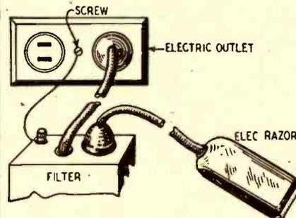
Fig. 2—Put line filters near the receptacle.
