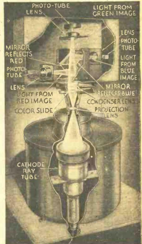
Photo D—Simultaneous system color analyzer.
