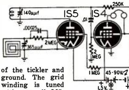
of the tickler and ground. The grid winding is tuned with a small 365- $\mu$ f variable. Plate voltages are supplied from a 45- or 90-volt B-battery, the latter supplying sufficient power for a speaker.
