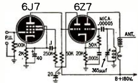
reduced by using a 20,000-ohm cathode resistor in this stage. The modulator section is connected as a cathode follower grid modulating the oscillator.
