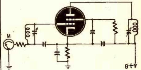
5. The above is a circuit of an r.f. amplifier. What is the fundamental difference between the action of the meter if the tube is operating Class C from what it would be if the tube was operating Class A?
