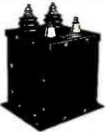
**Raytheon Pulse Transformer UX 4298 E.** Pri: 4 KV. @ 1 microsecond; secondary: 16 KV @ 16 amps. Filament pri: 115 V/400 cycles .....\$15
