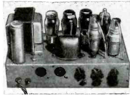
Fig. 3 (above)—The 6-tube, 13-watt amplifier. Fig. 4 (left)—Chassis layout of this unit.
