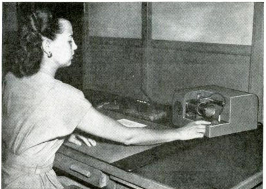
New Western Union facsimile machine brings the telegraph office to the executive's desk.
