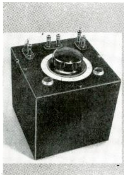
Fig. 2—Bridge is built in square steel box.
