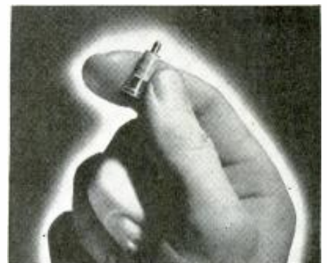
Fig. 3—Typical crystal for converter stage.
