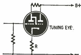
get current is much greater than the decrease in plate current so the total cathode current increases. The increase in cathode current through R biases the grid more negative, thus increasing the sensitivity of the tube and making the shadow angle smaller for a given grid voltage.
