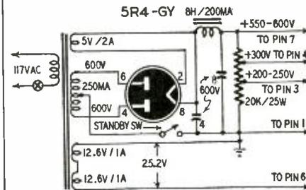
A. The components which you have should make an efficient power supply for the BC-696 or any of the other receivers in the SCR-274-N and ARC-5 command sets. The diagram is shown. The oscillator voltage may be reduced to 150.
