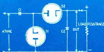
Fig. 1—The simplest form of doubler.
