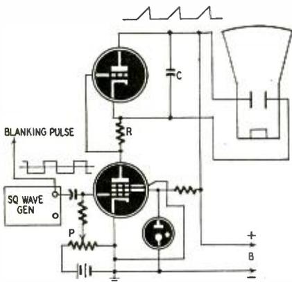
The pentode is biased below cutoff to conduct only when the square wave input exceeds its bias. The plate current of a pentode remains constant regardless of plate voltage. The screen voltage exercising considerable control over  $I_p$ , a VR tube is used to keep this voltage fixed.
