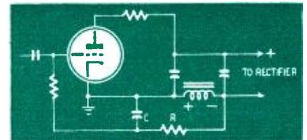
Fig. 13—Choke placed in negative lead.
