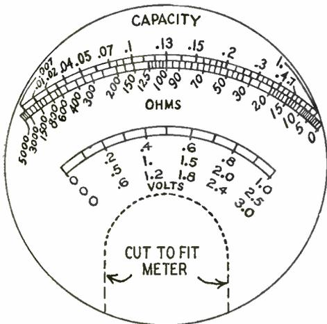
Fig. 3—Cut-out for the meter face. MAY, 1950
