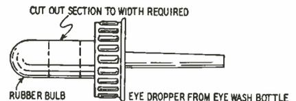
the bulb of a medicine dropper of the type which is built into the tops of eye-wash and nose-drop bottles. The rubber used in these droppers is of good quality, has fine grain and is of a convenient size.
