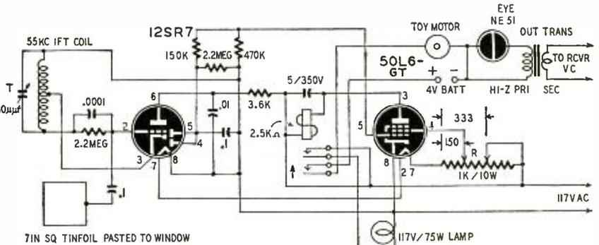
Body capacitance stops the oscillator to allow the 50L6 to operate the relay, which causes the Lucite figure's eye to wink, actuates a display and lights a sign.
