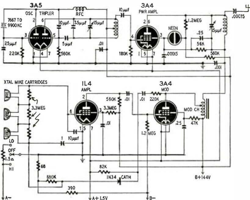
The r.f. section consists of a 3A5 Pierce oscillator and regenerative—overneutralized—tripler driving a 3A4 power amplifier. The antenna is a 20-inch length of thin aluminum tubing coupled to the transmitter through a spring-type loading coil. Measured output is 250 milliwatts.
