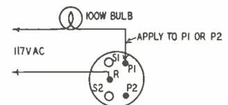
Fig. 16—Circuit for clearing points.
