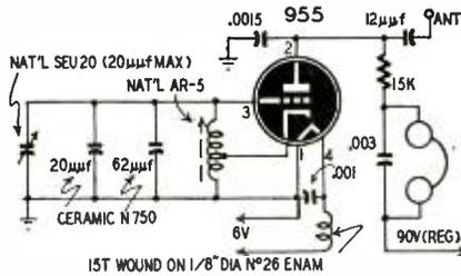
Fig. 2—Frequency meter for the unit.
