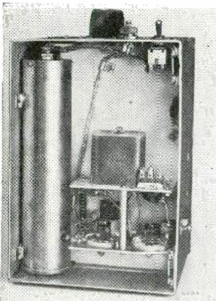
High-frequency section, internal view. The gold-plated coaxial resonator is at left and the 710-kc transformer near the center of the case. Below are the two 955 r.f. and a.f. oscillator tubes.
