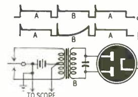
Fig. 10, left—Proper full-wave load balance. Fig. 11, center—Open at B upsets balance. Fig. 12, right—High-resistance joint in secondary unbalances current.
