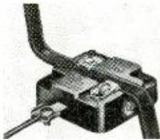
stamp of approval is a combination of the gap shunt-resistance types of arrester. It is easily installed under eaves, on a window sill, or on the wall; it can be used with all types of transmission lines but is primarily designed for use with 300-ohm, flat twin-lead. No stripping is necessary as toothed clamps on the arrester penetrate the insulation to make contact with the wires in the twin lead.
