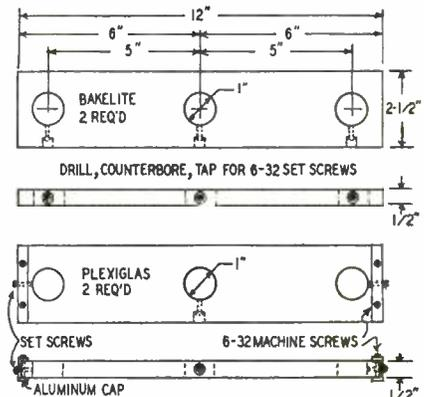
Fig. 2—Spacers for the triconductor.
