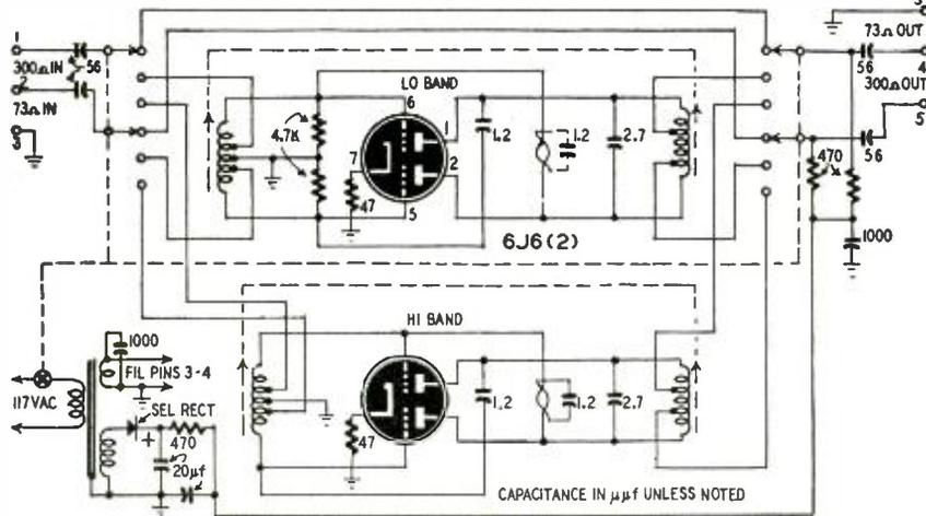
Fig. 4—The Regency DB-213. The 1.2-μf capacitors are simply twisted wires.
