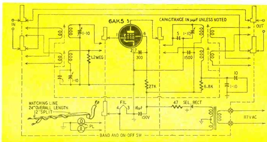
Fig. 1—The Anchor ARC-101-50 is permeability tuned on high and low bands.
