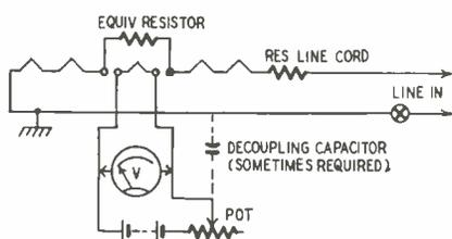
Fig. 1—Series heaters need resistor.
