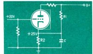
Fig. 14—R1 and R2 are voltage divider.
