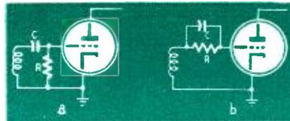
Fig. 10—Two circuits for grid-leak bias.
