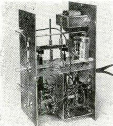
Two boosters use this smooth tuning system. Backlash is prevented by attaching the pointer directly to the tuning slugs.
