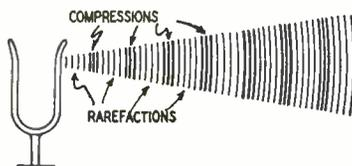
Fig. 1—Vibrating fork sets up waves. motion originally given to the first ball will travel through the whole string, causing each ball first to move closer to its neighbor and then to spring away from it.
