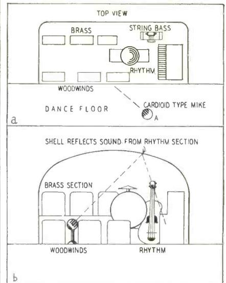
Fig. 2-a—Cardioid microphone facing orchestra at angle sometimes does best job. Fig. 2-b—Microphone in woodwind section picks up other instruments by reflection.
