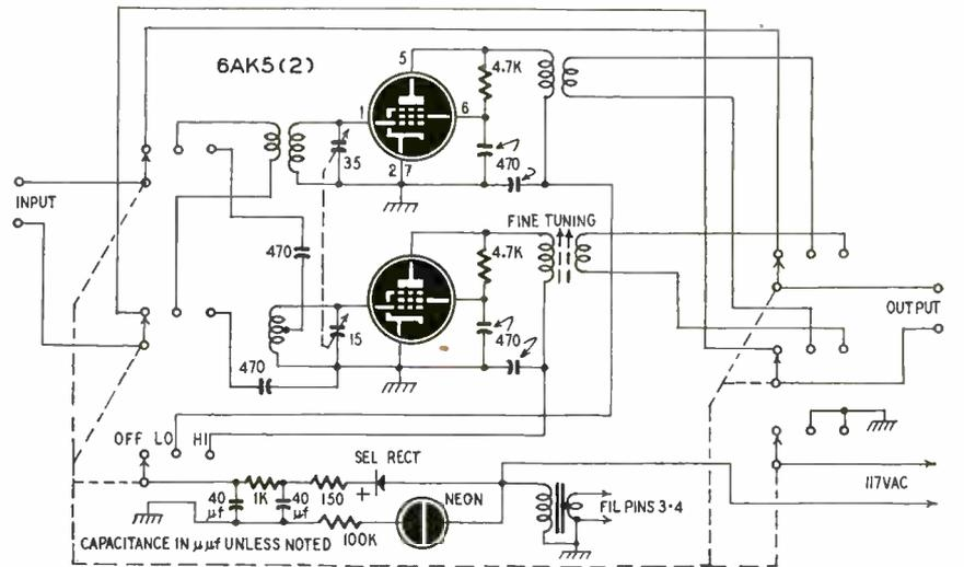
Fig. 3—High-band fine-tuning control peaks the permeability-tuned plate circuit.
