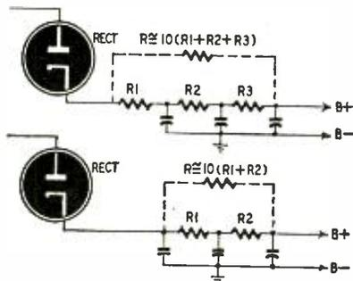
When R-C filters are used in B-supplies, the ripple voltage across the output capacitor is out of phase with the ripple voltage at the cathode of the rectifier. Resistor R delivers to the output capacitor ripple voltage which bucks out some of the ripple which passes through the filter. The combination of ripple voltages being less than the ripple voltage without R, the hum level is reduced.
