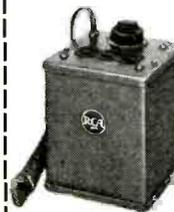
Eliminates shock hazard between ac/dc chassis and ground, speeds detection of receiver faults with high-low line tests, and facilitates testing at 117-volt design-center value. Has six-position primary switch and three secondary receptacles. Price: \$8.95.
