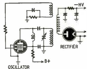
It consists of an r.f. oscillator whose output is fed through a step-up transformer to a rectifier. The output of the r.f. power supply can be filtered with relatively small values of filter components. This ease of filtering results from the low current drain and the high frequency of the ripple. Oscillator frequencies generally used are from 30 to 500 kc. Voltages as high as 5 to 10 kv are obtained directly with this type of supply.
