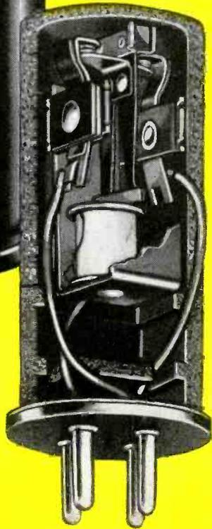
*Note rugged welded-steel box frame, mounting riveted elements rigidly and permanently in place. Only non-varying mica insulation used. No run-in required. Structurally stable—not unusual for 500-hour reading to duplicate initial values. Minimum contact impact and low contact-point erosion. Almost impossible for unit to close or stick. Heat generation low enough to sustain operation at 185° F.*
