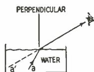
dense to a less dense medium, the light is bent away from the perpendicular. (An object at a appears to be, at a'.) In passing from a less dense to a more dense medium, the light is bent toward the perpendicular.
