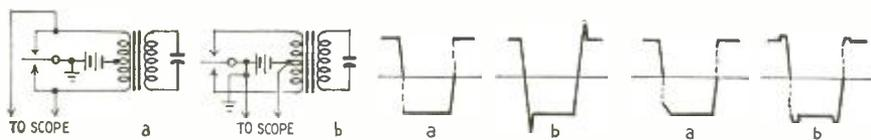
Fig. 7, left—Oscilloscope connections for waveform observation. Fig. 8, center—Non-synchronous supply waveforms. Fig. 9, right—Synchronous waveforms.
