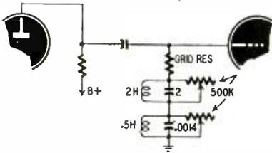
Fig. 1—Tuned circuits provide boost.
