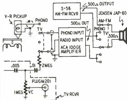
variable-reluctance pickup is connected to the phono input jack on the amplifier through the second pole on the TV-PHONO switch.
