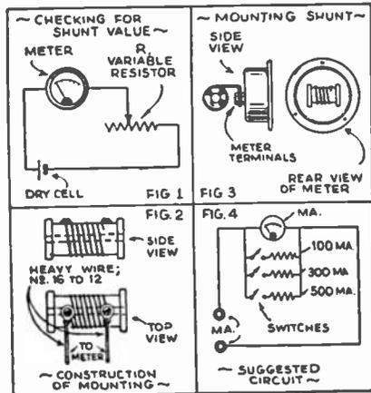
This cut-and-try method of determining the value of the shunt resistor can apply to any meter. For example, if a 10 ma. meter is to be arranged to read 50 ma., max. the reading during adjustment would be 1/5th of the full scale. One-fifth of 10 would be 2 ma., the scale reading to which the needle must drop back, etc.
