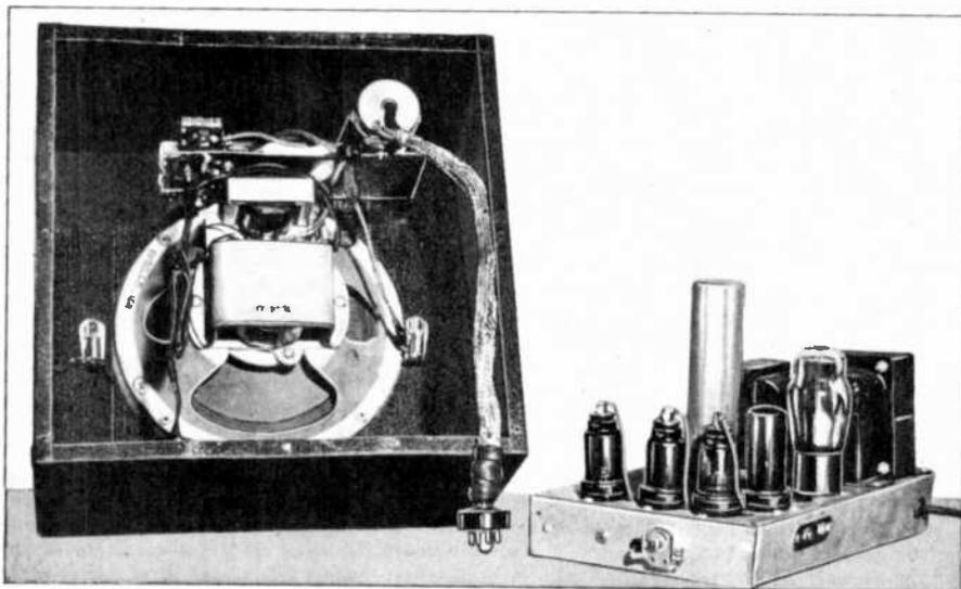
The rear view of test instrument shows the simplicity of its construction. Buzzer is on top shelf, at left of "eye" tube.
