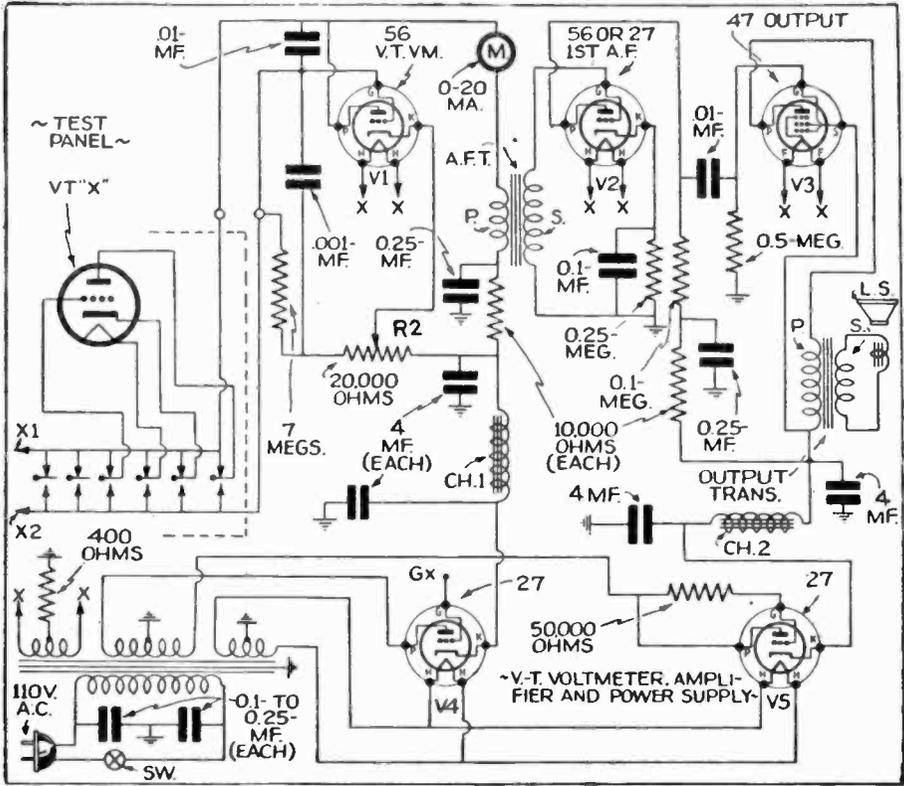
Fig. 1. Circuit of infinite-resistance tube checker.
