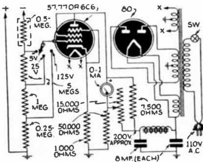
This unit is a direct-reading, 0-5-25-125V. D.C., V.-T. voltmeter with an impedance of nearly 7 megs. on all ranges. Another feature is the 0.5-meg. resistor
