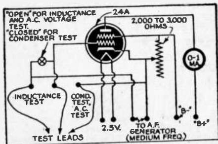
The calibration curve for inductances can be determined in a similar manner. When setting the meter at full deflection for inductance tests, the test leads should be shorted together. The switch should be set in the IND. TEST position.
