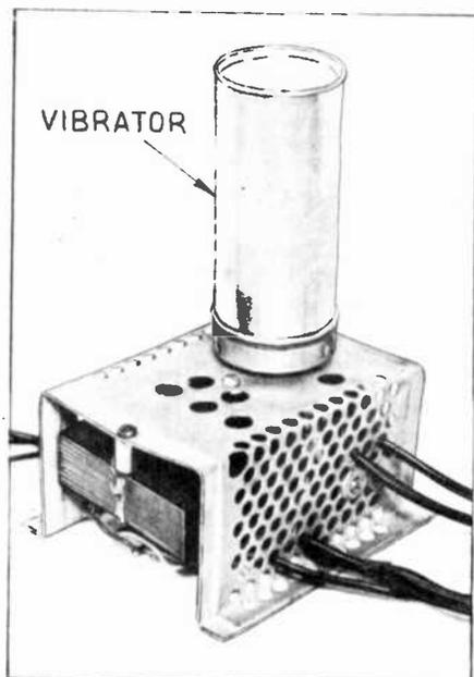
Completely assembled vibrator unit for obtaining from one cathode-ray tube practically the equivalent performance ordinarily requiring 2 such tubes. Many applications of this arrangement important to Servicemen are described
