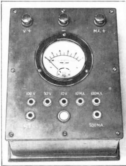
Fig. A. Photograph of the original model. Two additional range jacks, subsequently added, are included in the schematic diagram, Fig. 1.
