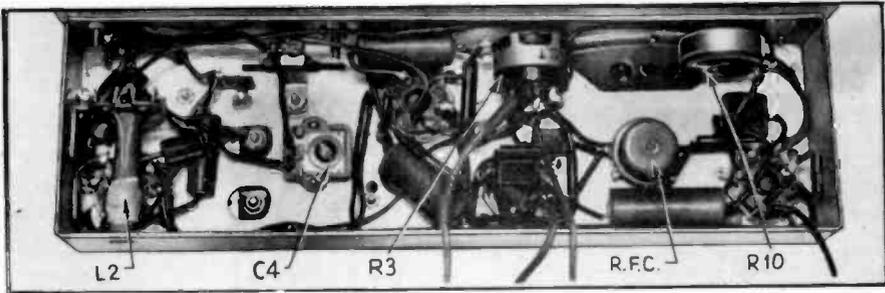
Fig. C. Under-chassis view showing the placement of parts and wiring.
