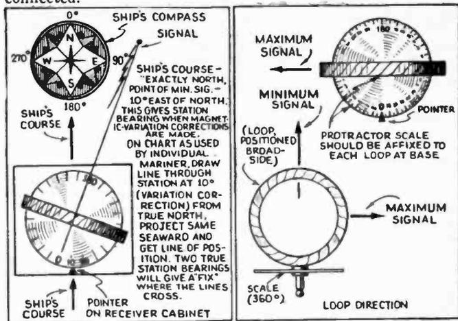
Fig. 1. Details of how the direction-finding loop antenna operates.
