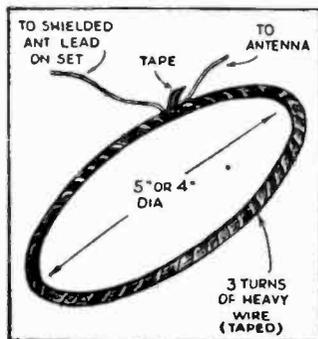
Noise-bucking pick-up coil for car radio.
