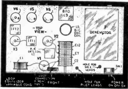
Fig. 2. Layout of parts on the chassis.
