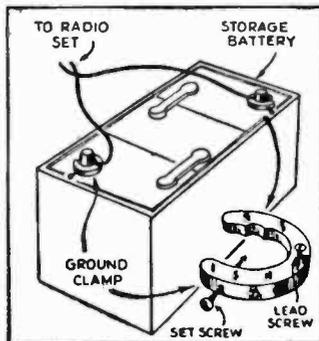
Ground clamp makes good battery terminal.
