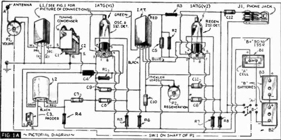
control is then advanced until the circuit is again just oscillating, and the I.F. transformer again adjusted until oscillation ceases. This procedure should be repeated until the primary and secondary are tuned to precisely the same frequency.
