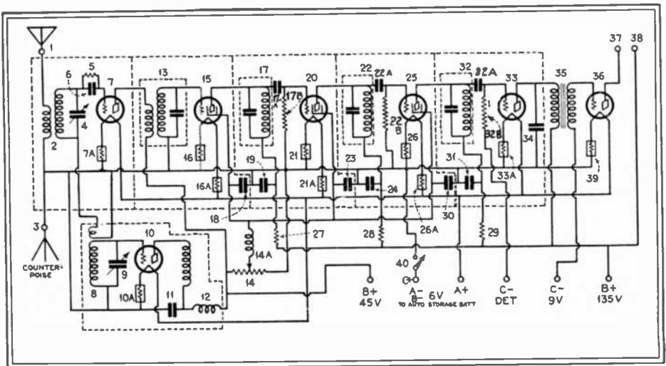
Fig. 59. Cisin "Screen-Grid" Automotive Superheterodyne. Complete details are appended.
