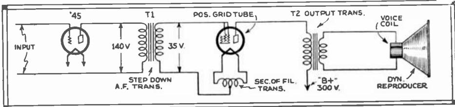
Fig. 100. "Class B Tube" Amplifier. The tube is a "46," designed to operate with zero plate current, under the "no signal" conditions. Note that transformer T1 steps down the voltage.
