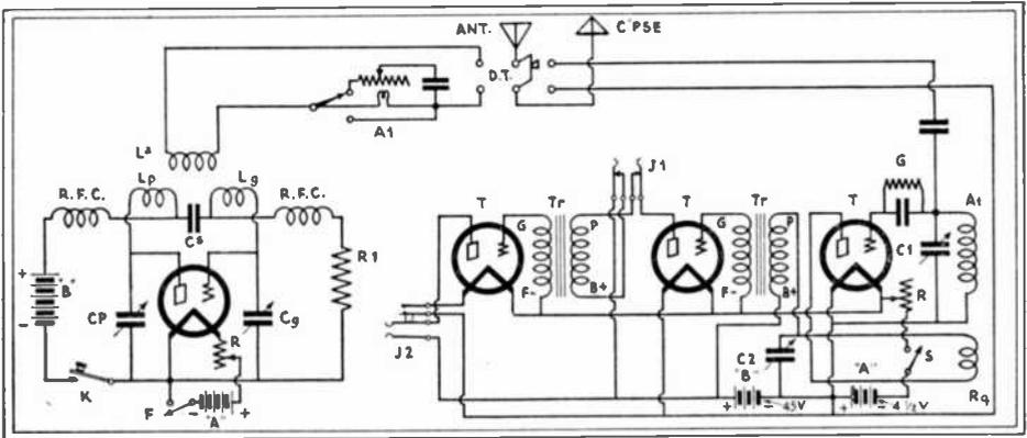
Fig. 74. A Complete Portable Transmitter-Receiver. Transmitter is a "Split-Colpitts."
