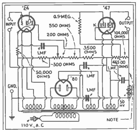
Fig. 67B, right. Type '47 Direct-Coupled Audio Power Amplifier.
