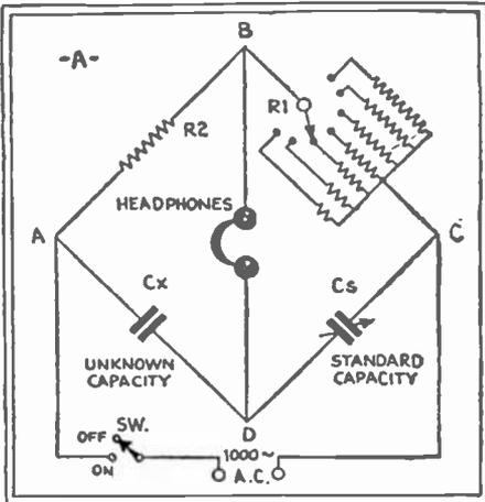
Fig. 97E. Wheatstone Bridge. Capacity.
