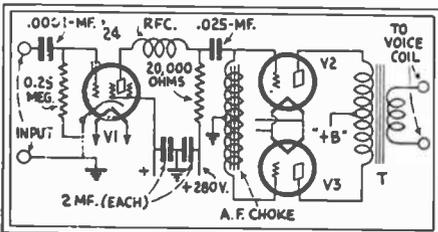
Fig. 89, left. High-Quality Detector-Amplifier Circuit. The output circuit is push-pull.
