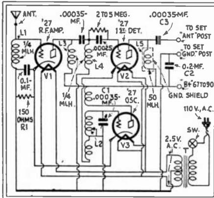
Fig. 55B. The Air-King Short-Wave Converter. Self-powered. A 2.5-volt transformer T supplies the "A" potential for the type '27 tubes used as R.F., det. and oscillator.
