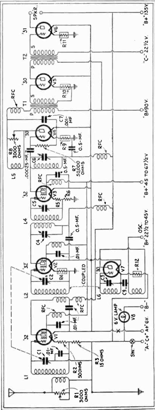
Fig. 28. A Superheterodyne Using 2-Volt Tubes. High sensitivity and "CW" reception are obtained by regenerating V4.
