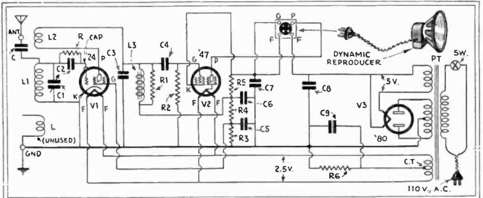
Fig. 2. The Radio-Craft A.C. "Pentode Portable." A Gen-Win 3-circuit tuner is used. The dynamic's field coil is the total filter inductance. Unit L3, 200 hy. or more. Fine experimental, regenerative circuit.
