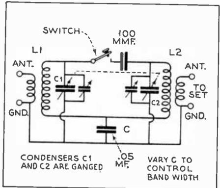
Fig. 88, above. A Band-Selector Unit. By varying the inductive relation of L1 and L2 control of the degree of band selection is obtained. Condenser C and the 100-mmf. unit further control the band selection.
