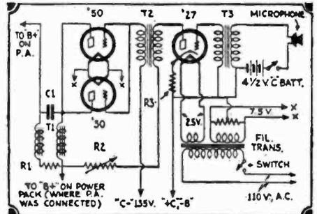
Fig. 98C. Transmitter. Modulator unit.
