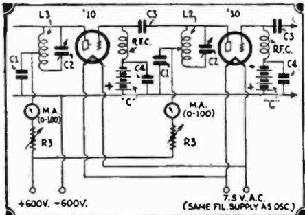
Fig. 98B. Transmitter. Frequency doubler.
