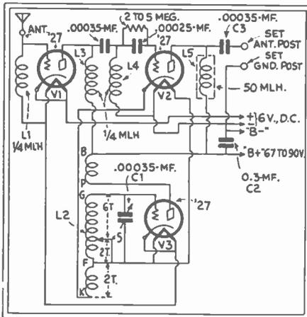
Fig. 55A. The Air King S.-W. Converter. A "Hi-Low" switch shorts 2 turns of L<sub>2</sub>.
