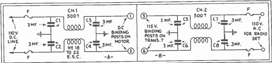
Fig. 75A, left: B, right. D.C. to A.C. Converter. Filters: A, input; B, output.
