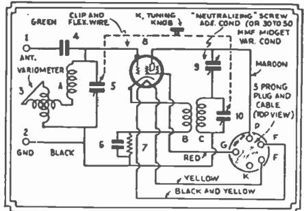
Fig. 51B. Police Converter—Cathode-Type.
