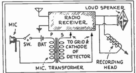
Fig. 62E, left; F, above, Recording. In Fig. 62 we find: A, connections for recording radio programs; B, circuit for recording voice, etc.; C, hookup for "home broadcasting"; D, reproducing recorded voice, etc. These changes may be switch-controlled, as indicated at E. Fundamentally, the circuit is very simple, as shown by the picture arrangement of the parts at F.
