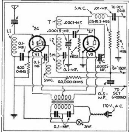
Fig. 53. A Screen-Grid S.W. Adapter.
