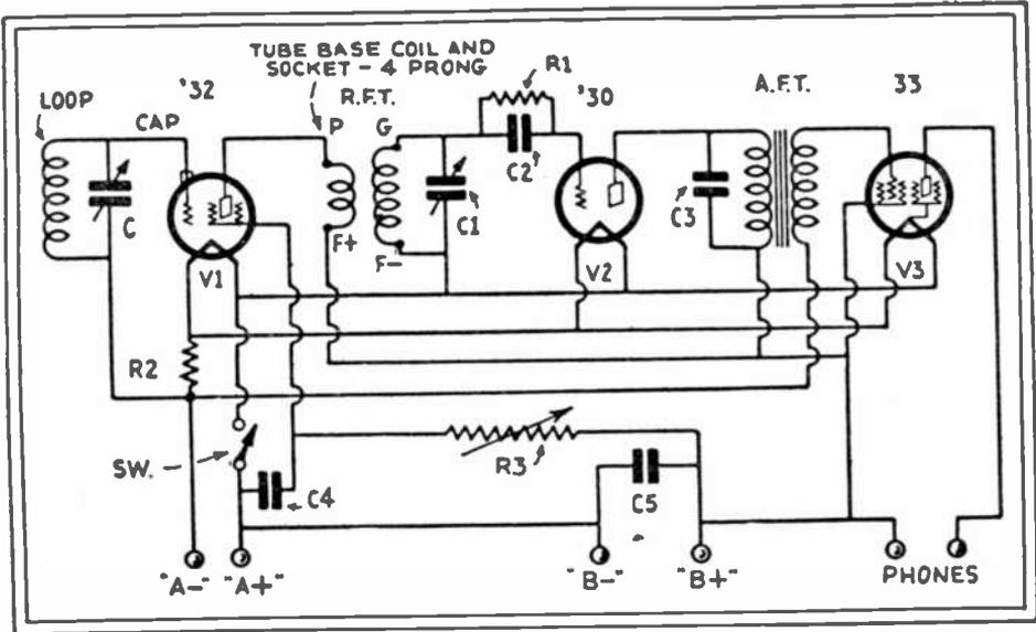
Fig. 93A. A "Treasure" Finder. The receiver; a simple short-wave set for 'phones.
