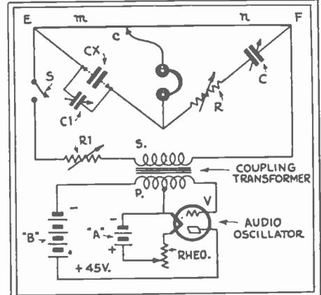
Fig. 97D. Wheatstone Bridge. Tube-type.
