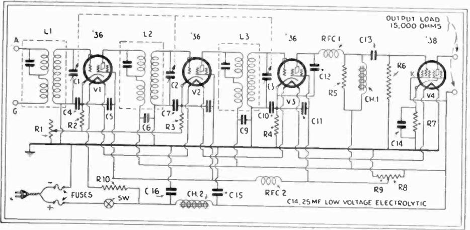
Fig. 5. A 110-volt D.C. Screen-Grid and Pentode 4-Tube Receiver. Note the use of a screen-grid tube as detector V3. Ballast resistor R10 must pass 0.3-amp. and drop to the 25 volts required for the four tubes in series; fortunately, the value is not critical. It is 283 ohms, for a 110-volt line, and 317 at 120 volts. Considerable amplification is obtained.
