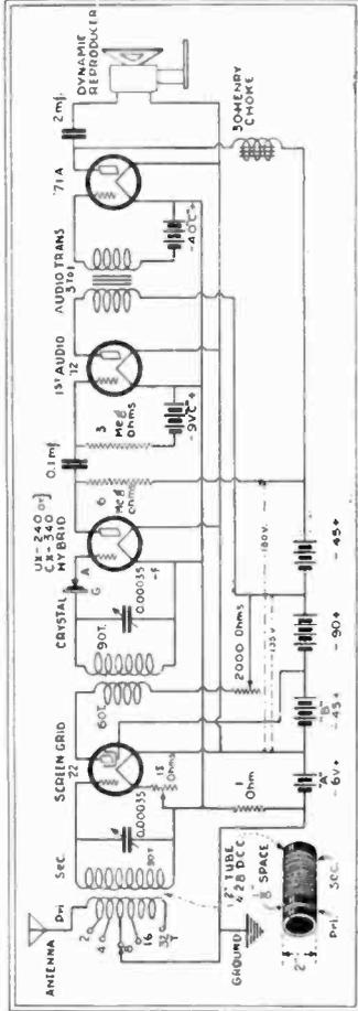
Fig. 30. The Grimes Hybrid-Crystal Receiver. Shield the '22 and second R.F. transformer.
