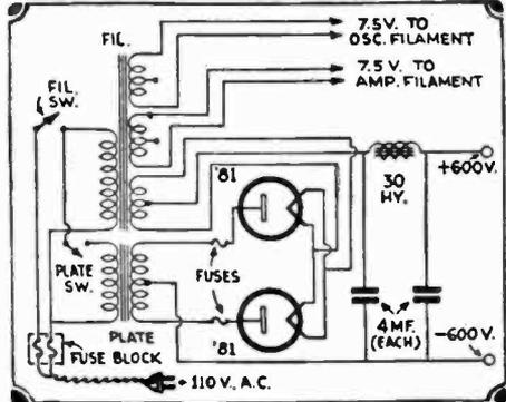
Fig. 98D. Transmitter. Power supply unit.
