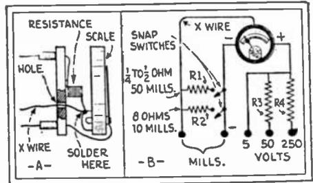
Fig. 94. Increasing A Meter's Range.
