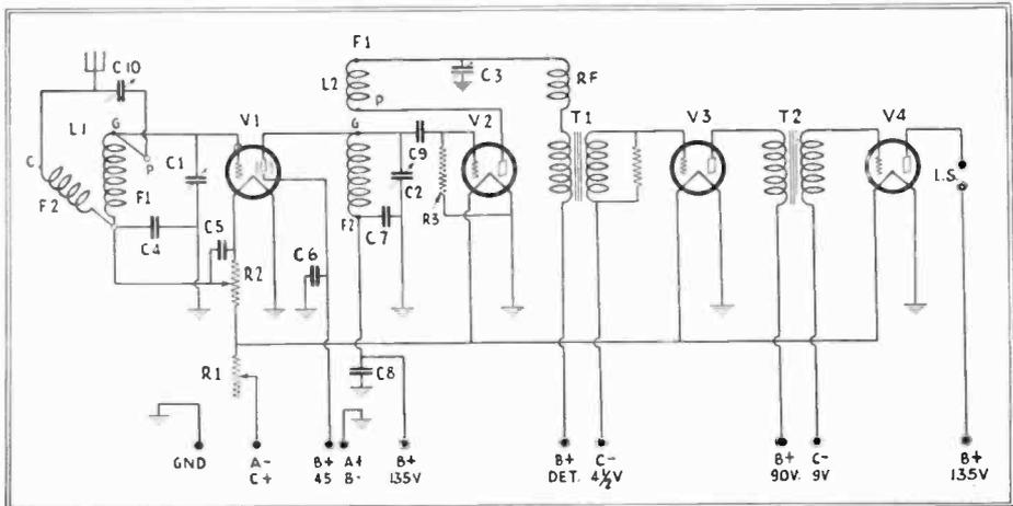
Fig. 48. The Pilot "Super-Wasp" Receiver. A complete receiver capable of reception from distant stations and at "loud speaker volume," so called. A very effective short-wave set.
