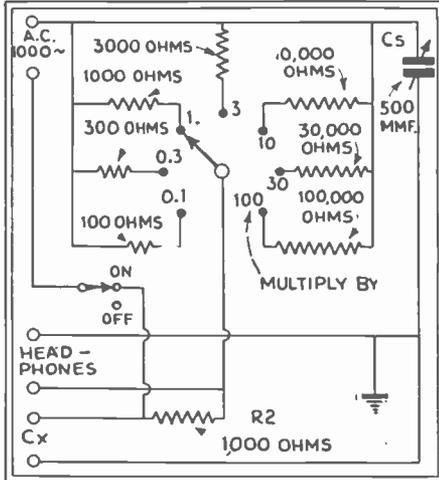
Fig. 97C. Wheatstone Bridge. Capacity.
