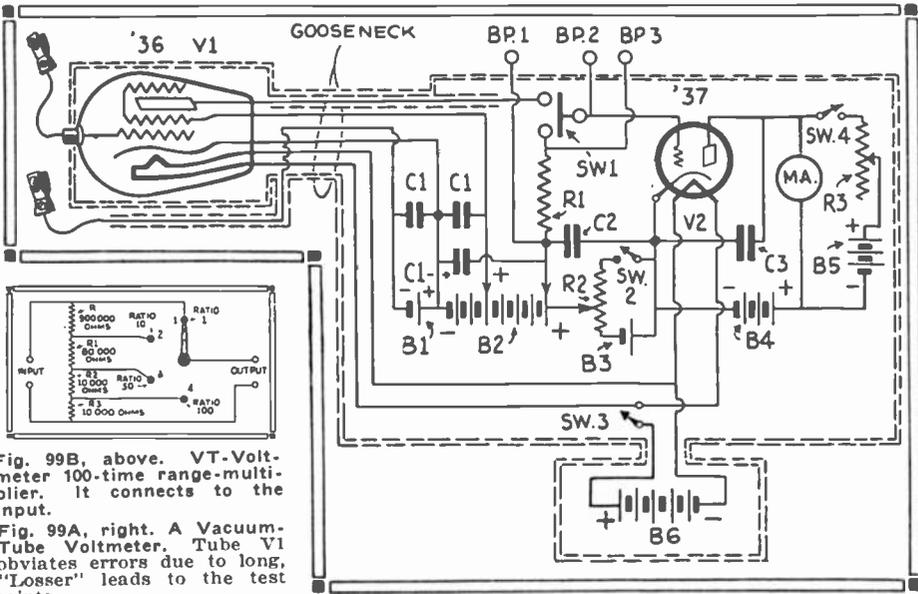
Fig. 99B, above. VT-Voltmeter 100-time multiplier. It connects to the input.
