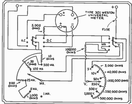
Fig. 86. A Wide-Range A.C.-D.C. Volt-Milliammeter. A general purpose test instrument.
