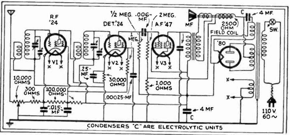
Fig. 6. The "Peter Pan" Model 84 Midget Set. Note the space-saving features: speaker field coil used as filter choke; resistance coupling between detector and power tube. Line switch and volume control are ganged. The output transformer must match V3.
