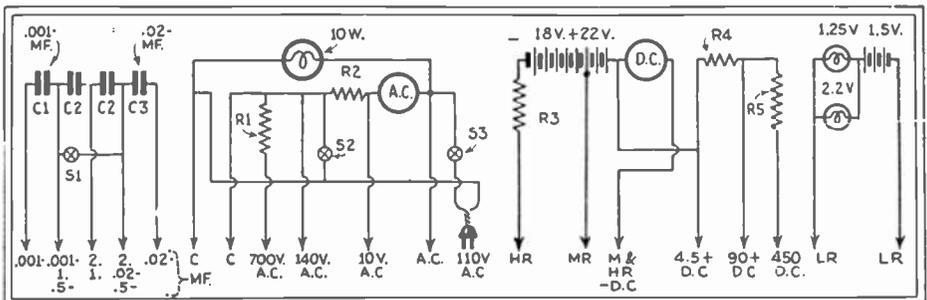
Fig. 92. An Inexpensive Test Panel. The wiring is simple, and the beginner should experience no difficulty with this design. May be used as an ohmmeter, continuity tester, capacity meter, and to read A.C. and D.C. voltages within the ranges indicated—and higher, if so designed. Arrowheads indicate tip-jacks. Condensers C2, 1 mf., each.
