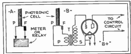
Fig. 82A. P.E. Relay Control—Photronic.
