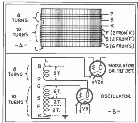
Fig. 55C. Air King Converter. Coil Details. The tickler and secondary windings of L, spaced 1/4-in., are No. 24 S.S.C. wire, on a tube 1 3/4 ins. in diameter.
