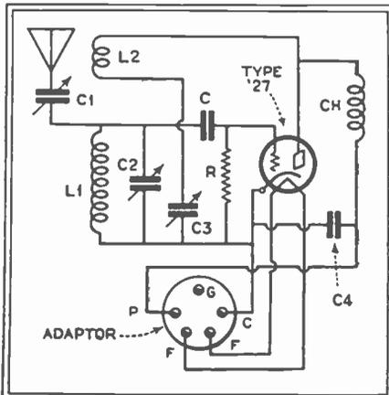
Fig. 52. An A.C. Short-Wave Adapter.
