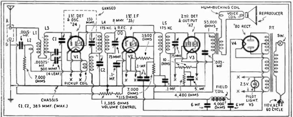
Fig. 3. Crosley "3-Tube" Superheterodyne. Type 131 "Tynamite" and "Bonniboy."
