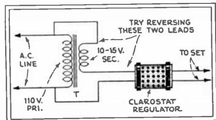
Fig. 84. Boosting Low Line Voltages. Reversing "sec." leads lowers line potential.
