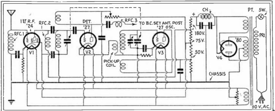
Fig. 54. The Walker "Model 4" Short-Wave Converter. A self-powered instrument.
