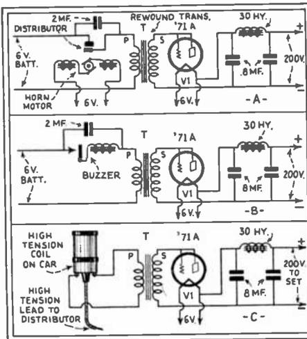
Fig. 95. Experimental D.C./A.C. Converters.
