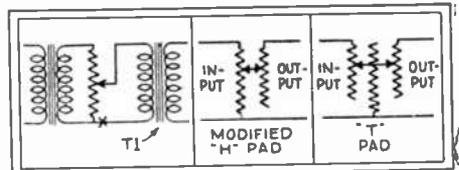
Fig. 81D. Mixing Panel. Types of pads.
