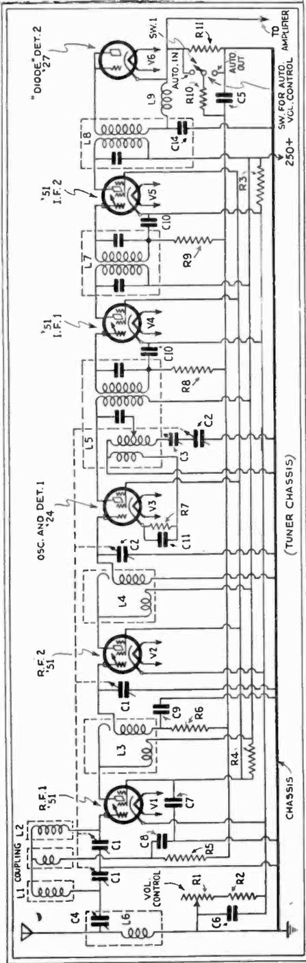
Fig. 33A. A Modern Superheterodyne Tuner Chassis—The Super-Da-lite-R. Readily adaptable to any power unit; includes A.V.C. and band-selection. To reduce cross-talk to minimum, type '51 variable-mu tubes are used in R.F. and I.F. Second-detector V6 is a diode.
