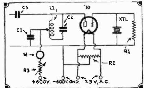
Fig. 98E. Transmitter. Oscillator hookup. When the five component units, A, B, C, D and E are connected together the ensemble is an up-to-date amateur phone and code transmitter—radio station W9DFR.
