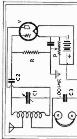
Fig. 29. The "B"-Less "Solodyne" Set. Plate potential for this receiver is obtained from the "A" battery. The coil is standard; grid condenser, .00025-mf.; grid leak, 2 megs.; P, 3,000 ohms; the tube, any type of triode.
