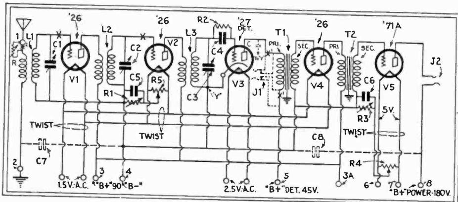
Fig. 12B. Circuit followed in electrifying the Freshman "Masterpiece," Fig. 12A, and other sets of similar design. "Electric" tubes are used as V1 to V5. A type '27' as V3 reduces hum; grid suppressors at X prevent "whistles." Resistor R may improve the operation.
