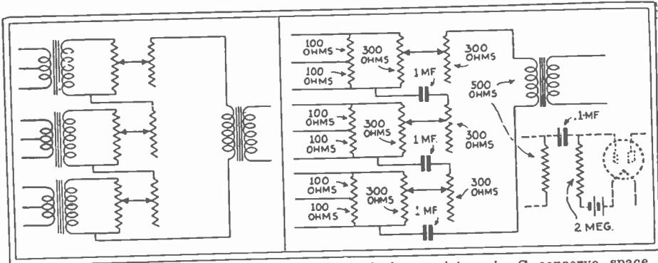
Fig. 81B, left; C, right. Mixing Panel. The 100-ohm resistors in C conserve space.
