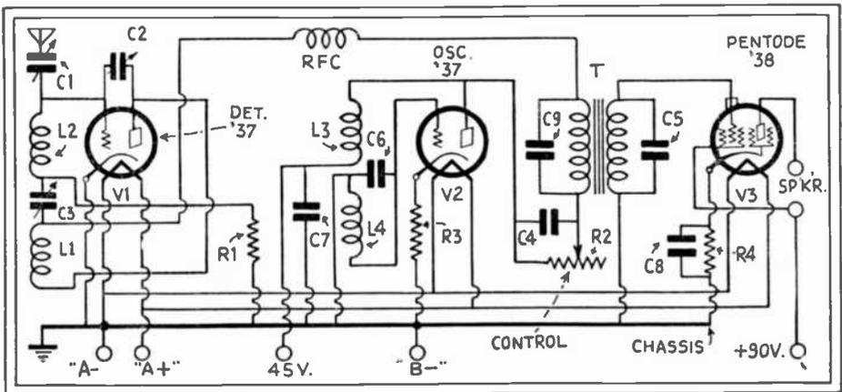
Fig. 39. A 5-Meter Superregenerative Receiver. A "quasi-optical" frequency set.
