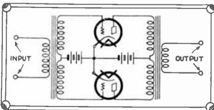
Fig. 68. A 1-Stage Push-Pull or Push-Push Amplifier. Whether the circuit is push-pull or push-push, depends upon the tubes and potentials. For push-pull action, use for "C" bias the potential shown in tables as correct for the tubes used. For push-push (class B, divide  $V_p$  by the tube's  $\mu$ ) to obtain the tube's grid bias for plate current cut-off; use Class B transformers.
