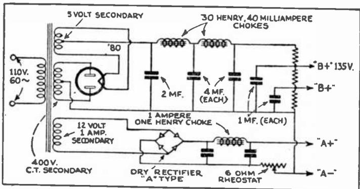
Fig. 35B. Power pack for the modern, simple All-Wave Set.
