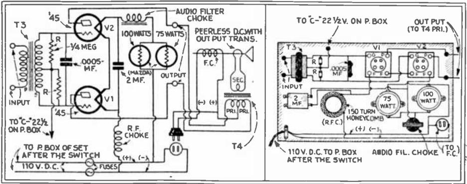
Fig. 66A, left; B, right. A 110-V., D.C. Audio Power Unit. At B, the parts layout.
