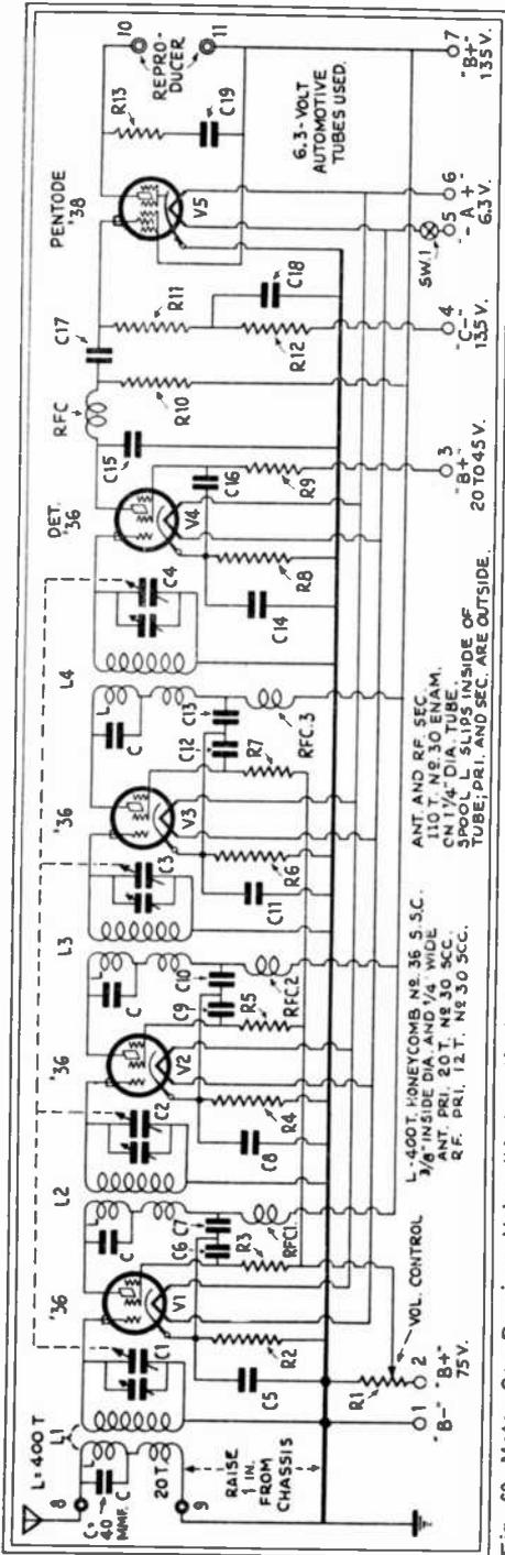
Fig. 60. Motor-Car Receiver Using "Automotive" Tubes. Four "comp ensated" R.F. transformers insure uniform sensitivity and selectivity.
