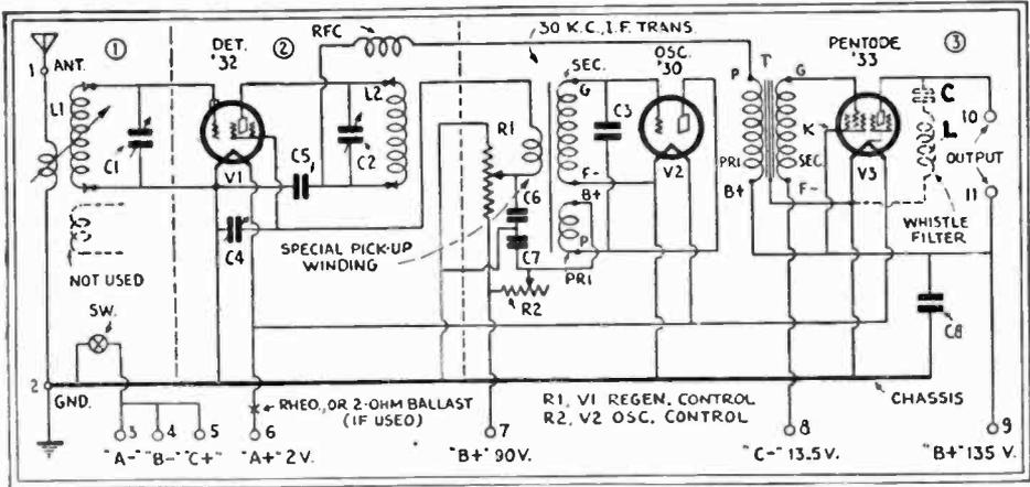
Fig. 46. The Short-Wave "Superregode"—With 2-Volt or "Dry Cell" Tubes. An ordinary 30-kc. I.F. transformer is used to obtain the super-audible suppressor frequency.
