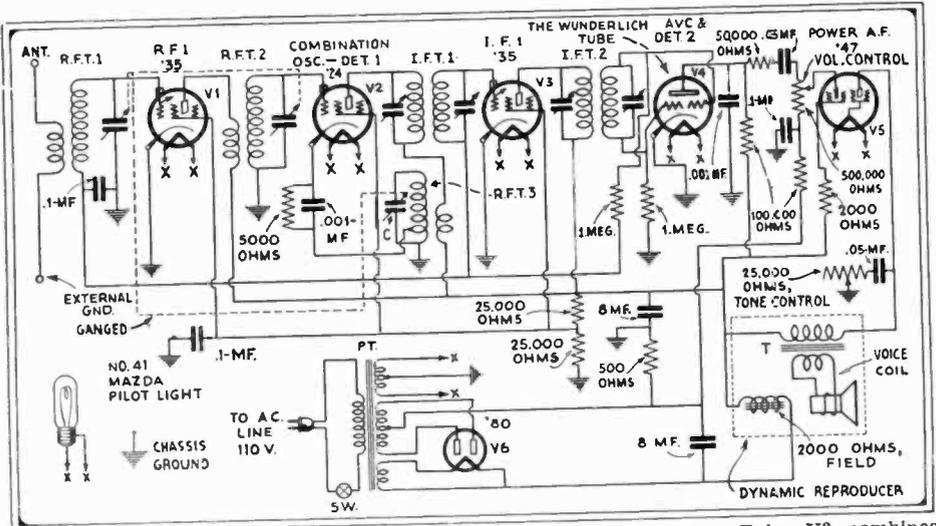
Fig. 8. An Ultra-Modern, Wunderlich-Tube, A.C. Superheterodyne. Tube V2 combines oscillator and first-detector; V4, A.V.C. and second-detector. This set is the Revere Model K2 chassis; the I.F. is 175 kc. Tube V4 is a "coplanar-grid" type Wunderlich "A" or "B."
