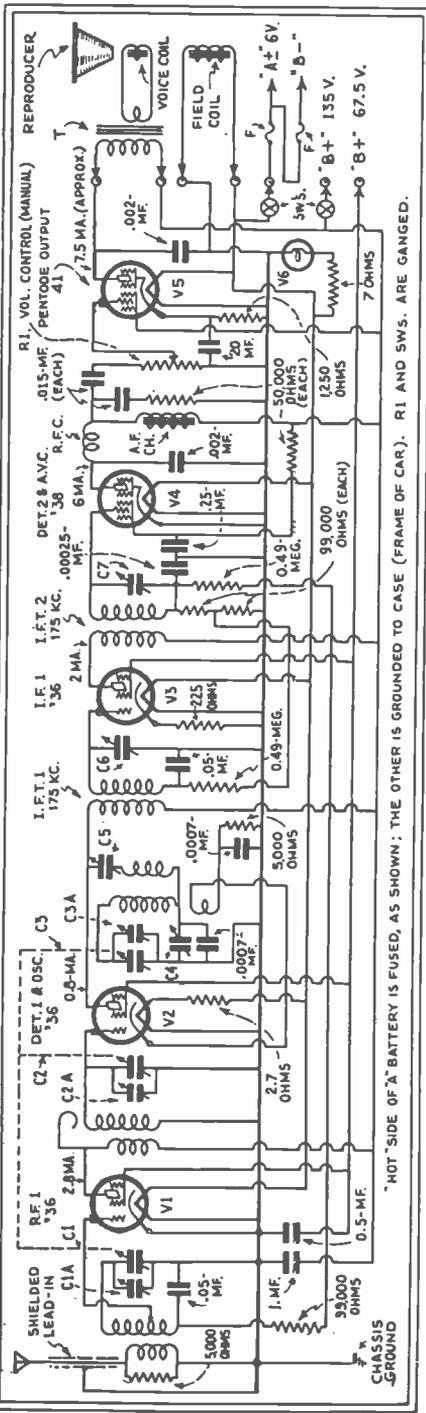
Fig. 61. The Philco "Transitone 7" A.V.C. Superheterodyne. Units C1, C2, C3, 325 mmf.; C4, 250 mmf.; C5 to C7, C1A to C3A, 50 mmf.
