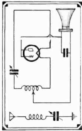
Fig. 34. A Batteryless Tube-Type Receiver. The '71A filament receives its power from the broadcast station, which must be a high power local. The secondary coil is 3% in diameter and 2% in long; No. 22 D.C.C. wire, primary, (wound with bell wire), and condenser, experimental. Tuning condenser, 0005-mf.; the speaker bypass, 0.25-mf.
