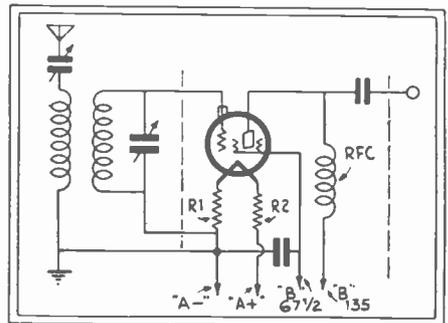
Fig. 80. A Screen-Grid Booster Unit. The tube may be any type suited to the set.
