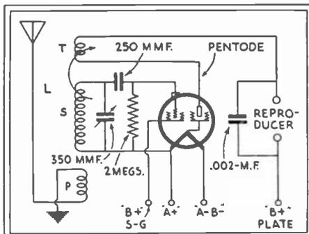
Fig. 14. A 1-Tube Pentode Receiver. For broadcast wavelengths, the grid-leak and grid-condenser may have the usual value, respectively, of about 2 megs. and .00025-mf.; for short-wave reception, over 3 megs. and below .00015 mf. A standard 3-circuit tuner and tuning condenser are used in this set-up. Although a battery-type tube is shown, considerably greater output would be obtained from an A.C. tube. The plate voltage will depend on the individual tube.
