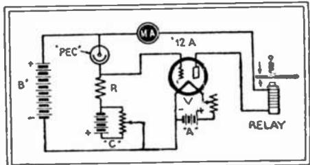
Fig. 82C. P.E. Relay Control—Gaseous.
