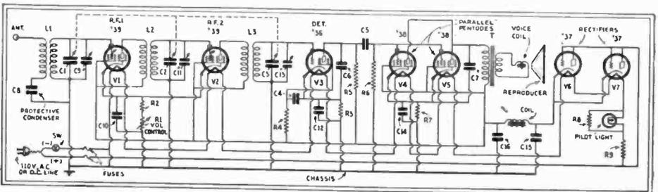
Fig. 7. A Modern A.C.-D.C. Pentode Portable Receiver. Two type '37 tubes, with the elements in parallel, furnish adequate rectification on A.C. circuits; on D.C. they act merely as a series resistance. Tubes V1 and V2 are variable- $\mu$  R.F. pentodes. Use no ground.
