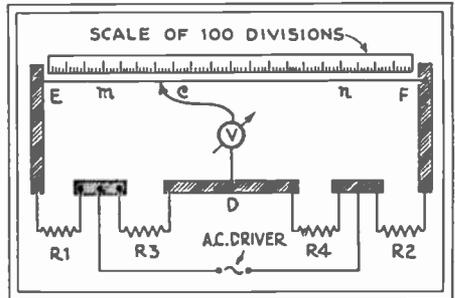
Fig. 97B. Wheatstone Bridge. Meter-rule.
