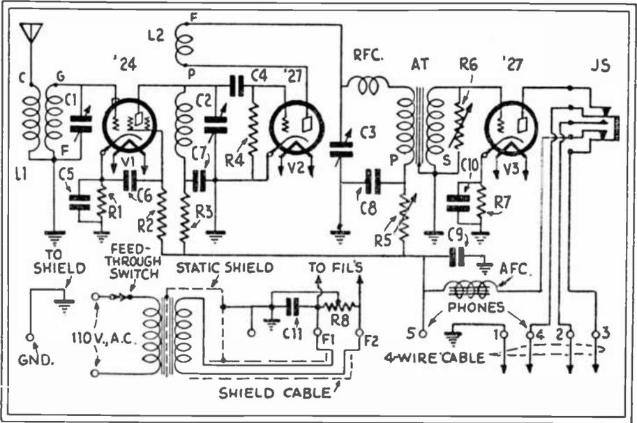
Fig. 50. A Short-Wave Adapter-Receiver. An R.F., detector, and A.F. combination.
