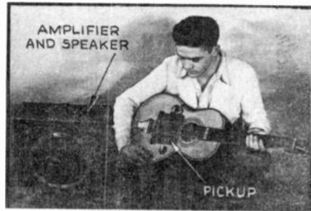
Every orchestra should have at least one electronic music instrument in its ensemble. Mr. Kendall Ford's unique pickup may be used with any steel-stringed instrument.
