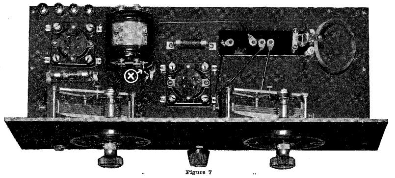
for the C battery added later. Where it passes the underside of the second binding post from left, connect it to that post by a short length of wire. By these operations we have completed the positive circuit and can begin on the detector cir-
