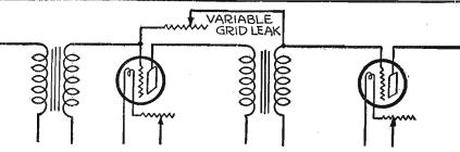
If you are troubled with various unvanted noises, try out this simple little experiment. In the accompanying sketch experiment. I show where an ordinary variable grid leak is connected between the grids of the last and preceding audio frequency tubes in order to control various kinds of distortion. I have found this arrangement most satisfactory. The resistance should be set at its lowest value and then
