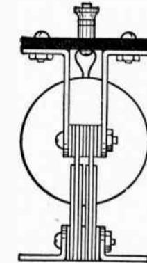
The view above shows the method of assembling the transformer
