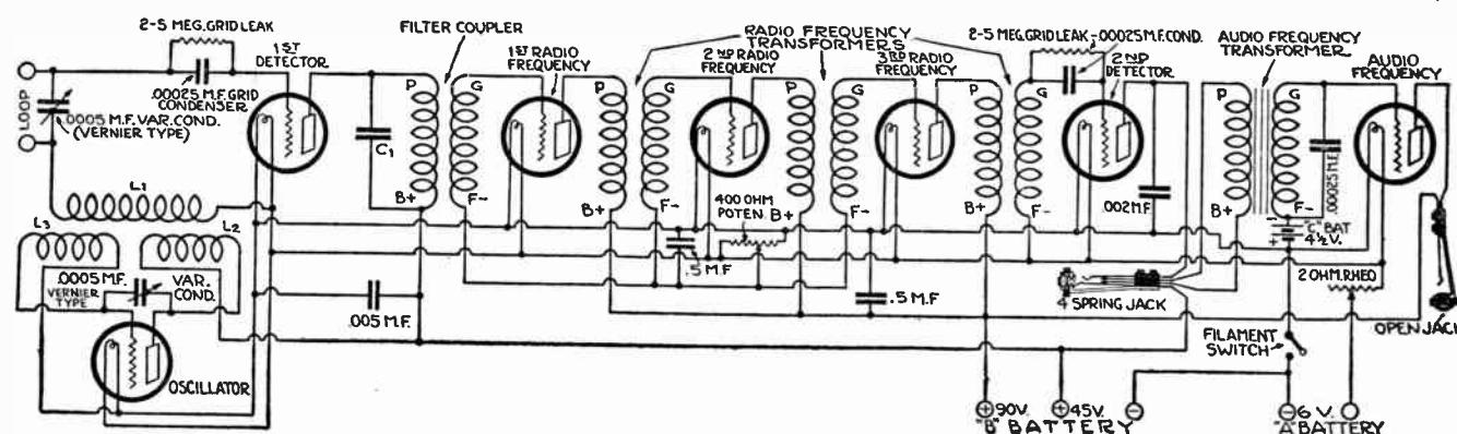
plete and that the B battery circuit is not connected in any way that it will blow out the tubes. Now turn the filament switch off, insert the remaining six tubes and again turn the rheostat to the right. All this was done previously of course, but this second preliminary test is desirable to be sure that connections made since the first test have not been made so that the B battery will blow tubes.
