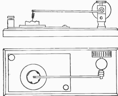
Figure 2—Details of Detector Stand
