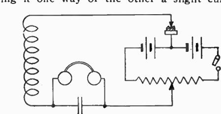
Figure 4—Circuit Employing Potentiometer and Local Battery
