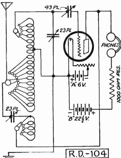
It is suggested that the three condensers be placed on the horizontal center line of the panel, one being close to the left hand edge, the other two close together at the right hand edge. Switches are then placed slightly to left of center between condensers one and two.
