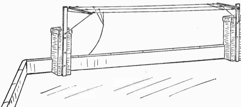
Figure 3—This three-wire inverted L utilizes two chimneys as anchors for short two-by-fours
