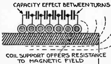
Figure 1—Detail of cross section of plain inductance showing source of losses
