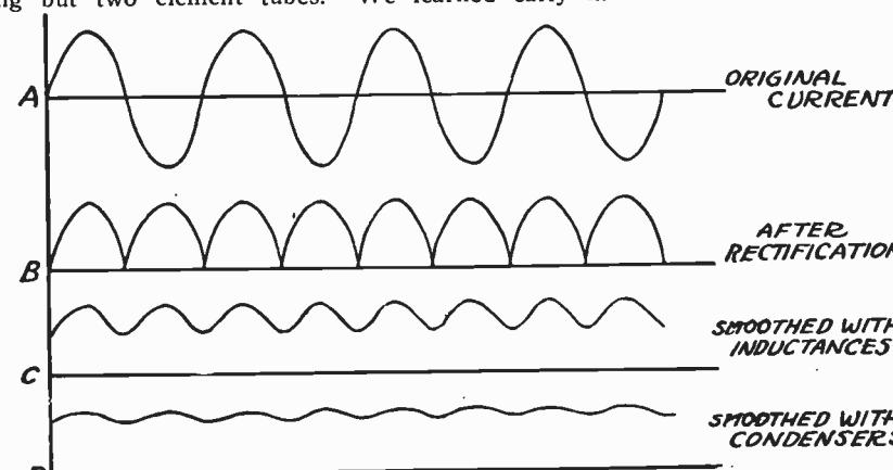
Figure 230—Showing various stages in converting A. C. to D. C. for use in plate circuits
