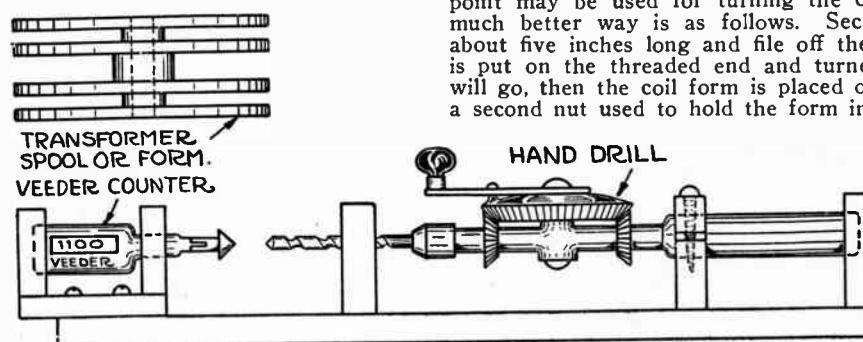
illustration shows a way in which coils may be wound for the Radio apparatus by the application of this drilling tool.
