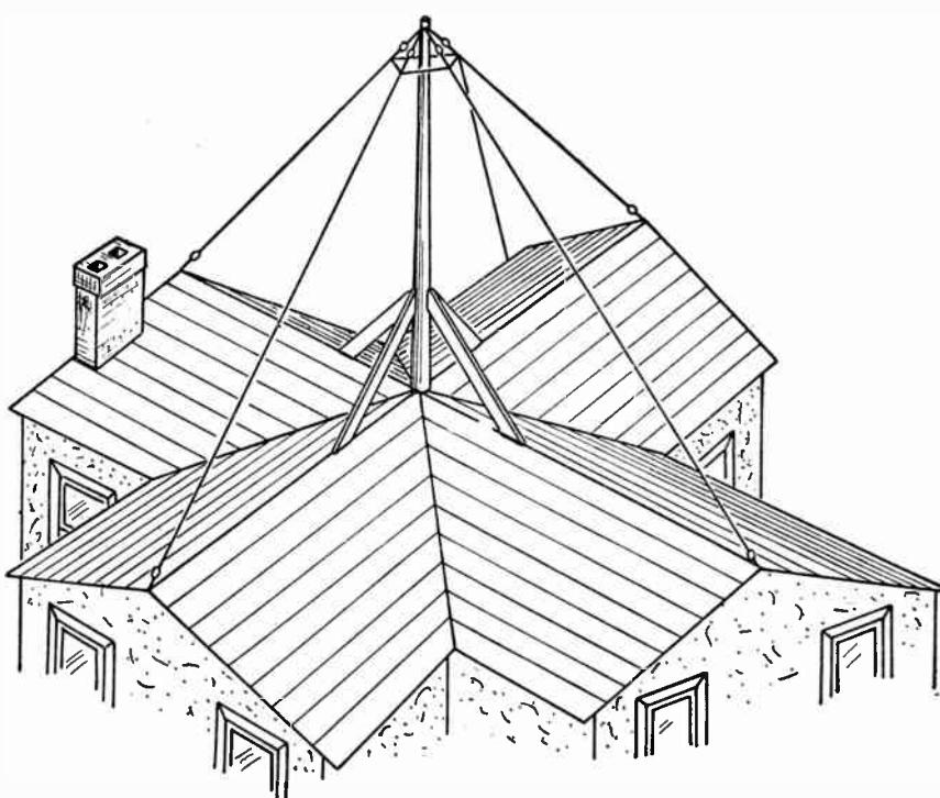
Figure 7—The umbrella aerial used where large area cannot be obtained
