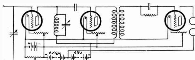
Figure 2—Two stage amplifier using tuned coupling and transformer
