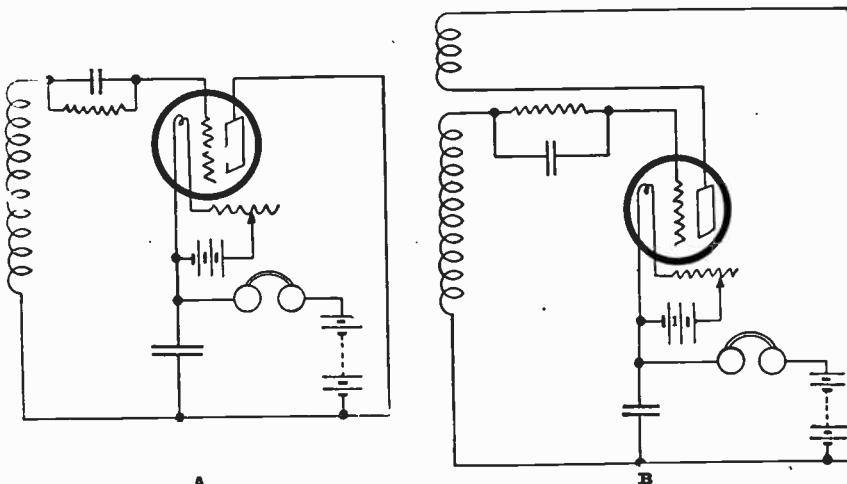
Figure 227—Analysis of Flewelling circuit to show principles of operation
