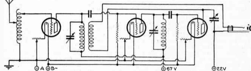
Figure 240—Regeneration includes not only detector but a step of R. F. amplification as well.
