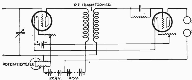
Figure 1—One stage of Radio frequency amplification coupled to detector
