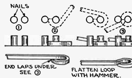
ing them just far enough apart so that the ends of the wire may be slipped between them. Place the end of the wire against the side of one of the nails; it then becomes easy to bend the wire around the other nail, making a uniform loop.
