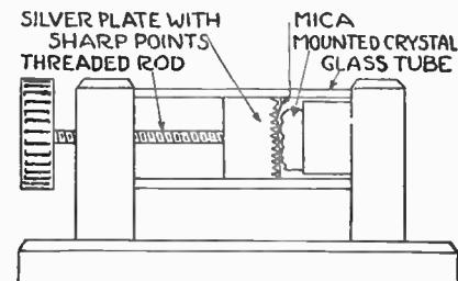
Figure 3—Detector Stand for Iron Pyrites
