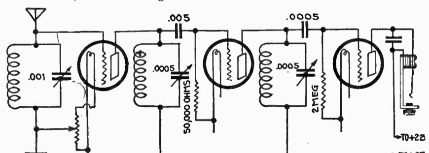
Figure 232—Two stages of tuned impedance coupled Radio frequency amplification
