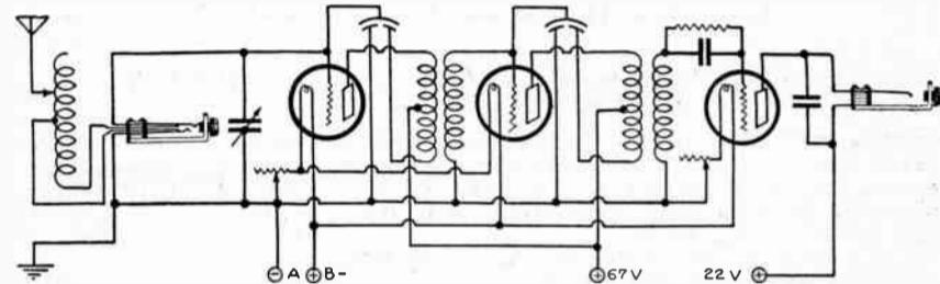
Figure 239—The tubes are prevented from oscillating by splitting the primaries of the transformers and introducing small condensers.
