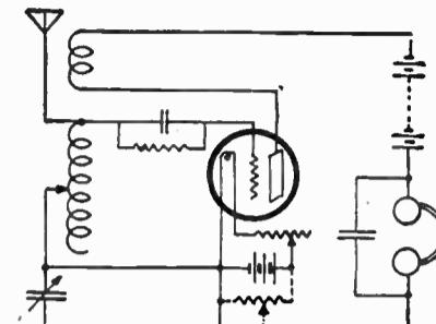
Figure 5—Conventional Single Circuit Using Tickler Feed Back
