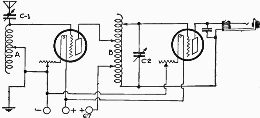
Figure 234—The French amateur's equivalent of the American "ham's" Reinartz—the Abele
