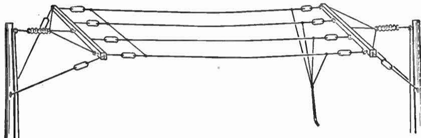
Figure 1—The four-wire inverted L is probably the most popular type.
