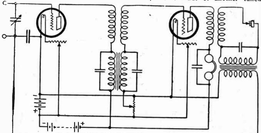
Figure 222—Circuit using transformers for both Radio and audio coupling
