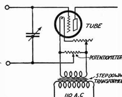
Figure 228—How A. C. is used in lighting filament
