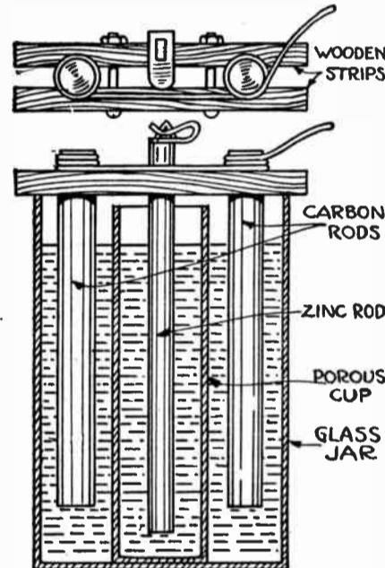
Figure 2—Converting sal-ammoniac cell to bichromate cell.
