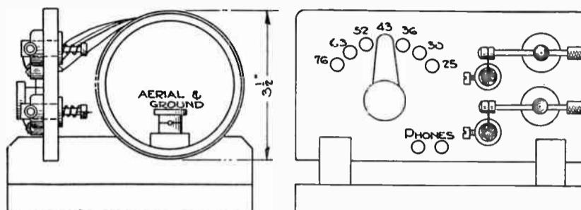
Each crystal detector consists of a central pivot drawn in by a spring, a cat-whisker stem slidable through a transverse hole in the end of the pivot, and
