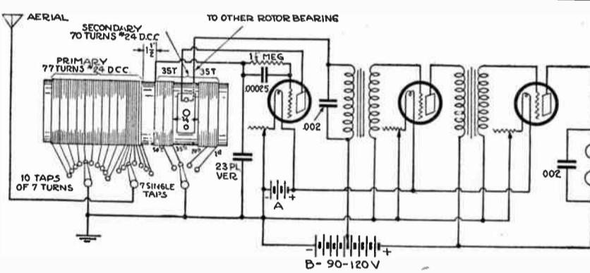
pins and the bearing plates on the tube. Solder the outside or end wires of the rotor on the shafts. This may look like a big job, but if description is followed it will not take long to finish it and you will find it worth while. A better tuner cannot be made. The controls should all have vernier adjustments.
