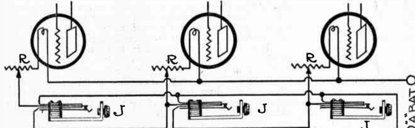
This device is a great saving on batteries because sometimes a person desires to listen in on one or two tubes on a three tube set. Without a jack the third tube must burn and at the same time the listener does not get any use of it, it only draws power from the battery. The rheostats can be turned down but think how simple it is just to change the plug to another jack and not have to touch a control knob. The illustration is clear enough to be understood without further explanation.
