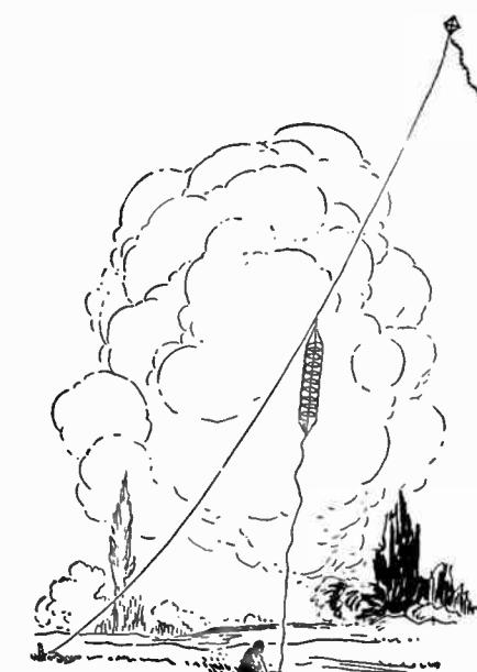
Figure 12—The spiral elevated by a kite for use with portable sets.
