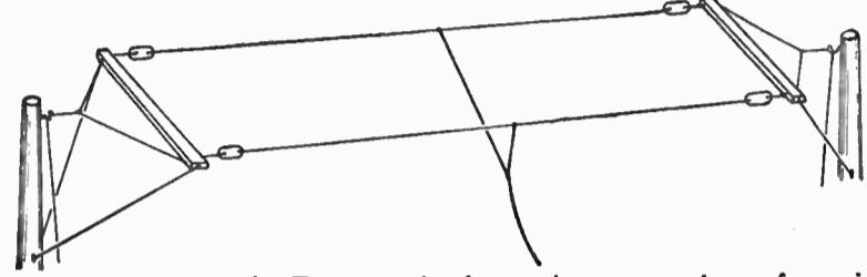
Figure 4—The two-wire T-antenna is often easier to erect than a four-wire inverted L.
