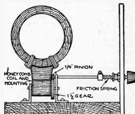
gearing and knob insulated from the circuit. A friction spring is used to hold the coil in any position that it is set. I use the gearing arrangement on the tickler coil in order to make the well-known grid circuit as short as is possible. The tickler coil has pigtail connections.
