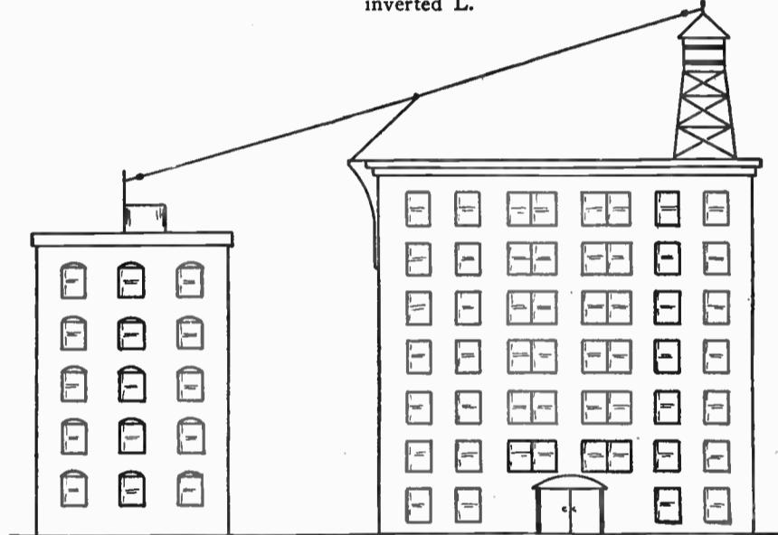
Figure 5—The single wire T, in this case, is less unsightly than a multi-wire inverted L would be.
