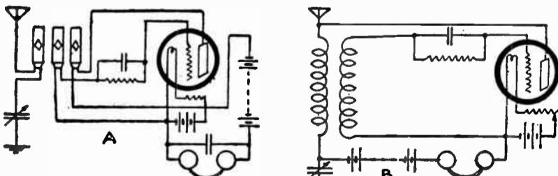
Figure 3—Tickler Feed Back as Applied to Two Circuit Tuners. (Not Advised.)
