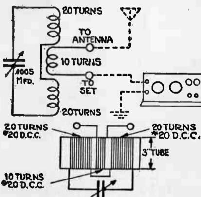
Figure 3—Inductively Coupled Wave Trap
