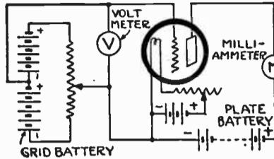
Figure 2—Circuit to Determine Characteristics of Vacuum Tubes and Demonstrate Effect of Inserting Control Element Between Filament and Plate
