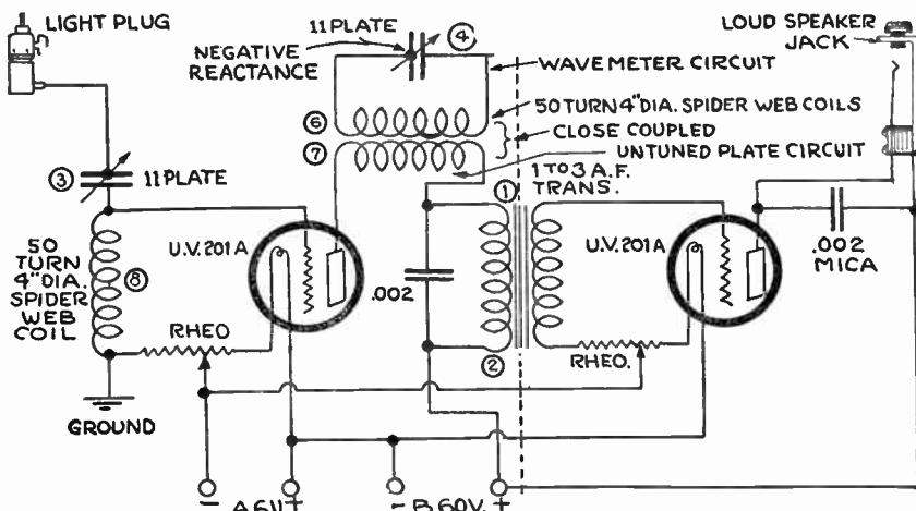
set operates well on an indoor lighting socket plug, with input to loud speaker of Magnavox type. The aerial condenser and coil should be located at least
