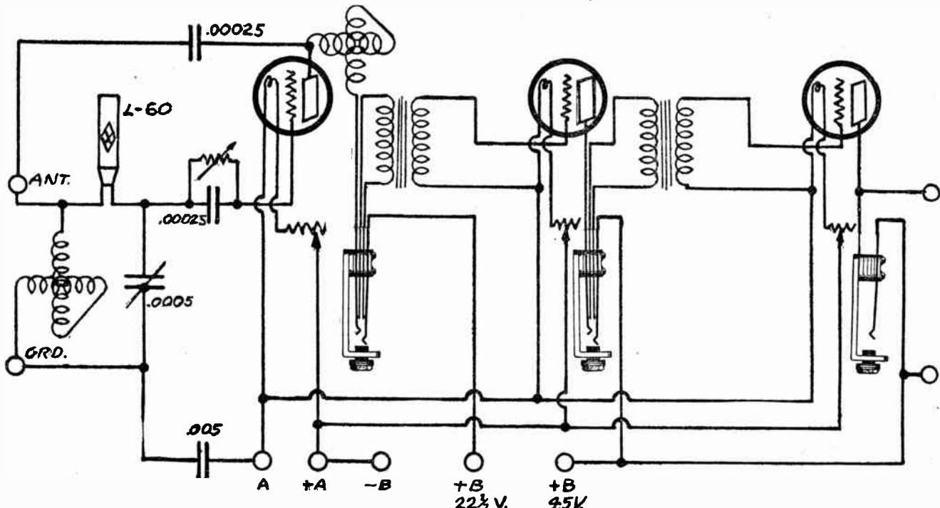
plate battery voltages can be varied by experimentation for clearest reception and maximum volume.
