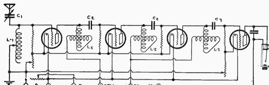
Figure 238—Type of tuned impedance R. F. amplification designed by Leon Bishop, 1XP.
