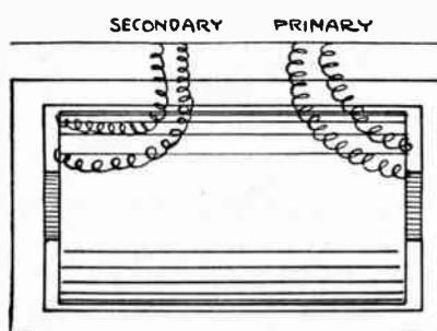
core—out of both; and keep the core—the bunch of annealed wire in the center. If you want to know how many layers are on a coil count them. It's good practice. On most coils there are 35 and 37 layers. If we have a 35-layer coil and desire a 10 to 1 ratio it is necessary to have a 30 to 3 coil.
