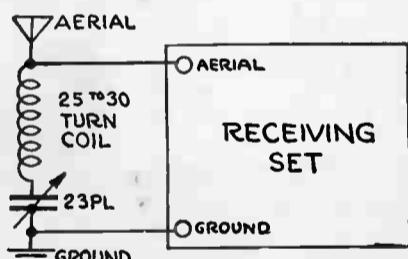
Figure 2—Parallel Type of Wave Trap
