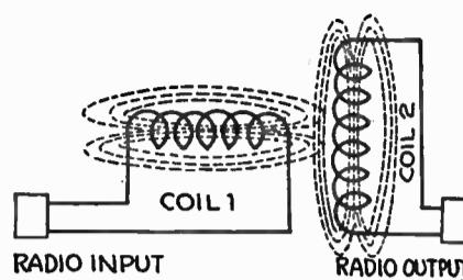
a weak or negligible current is set up in the second coil by current through the first one.
