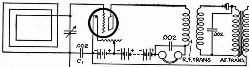
Figure 220—Simplest form of one-tube reflex to show principles of operation
