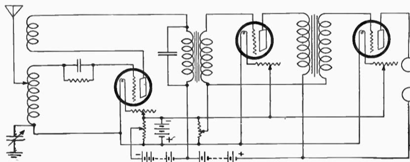
Figure 2—A fully developed circuit for two stage audio frequency amplifier
