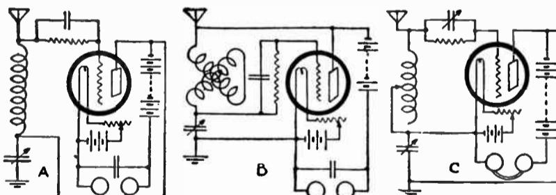
Figure 2—The True Ultra Audion Circuit and Two Modifications
