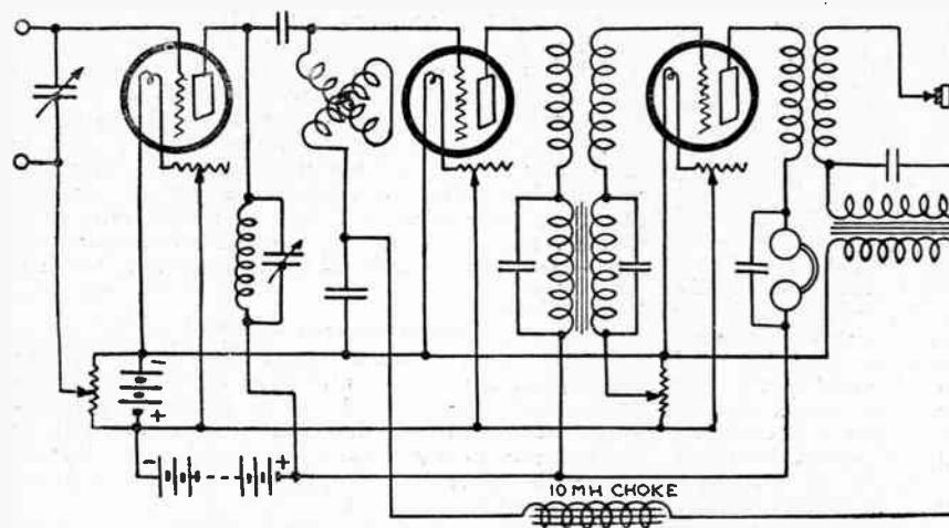
Figure 223—Three tube reflex using tuned Radio frequency amplification
