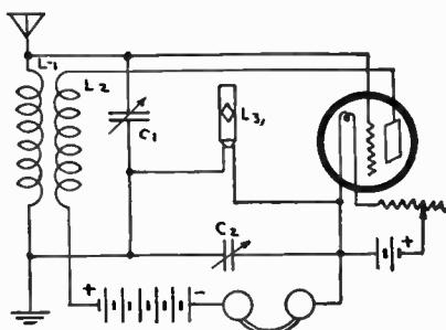
THIS hook-up is a new single tube receiving circuit, known as the Nacireman. This circuit was developed in the laboratories during a series of experiments with a large number of receiving circuits. This new circuit is not suitable for wired Radio because of its tendency to reradiate, but it is probably the last word in a simplified single tube set for receiving news and music from the present Radiocasting stations.
