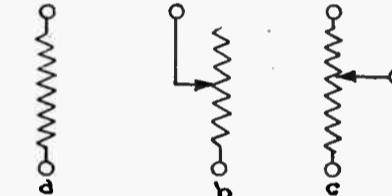
Figure 5—Resistances are shown in these drawings, one fixed, one variable, one of a special unit
