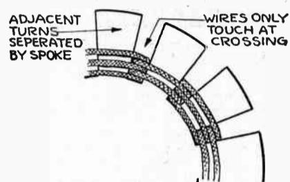
Figure 2—Detail of spider web showing how distributed capacity is reduced by increased spacing between wires
