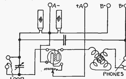
Figure 226—Diagrammatic circuit for one tube super results. The small tubes using 1½ volts on the filament will work, but the larger plate currents possible with the larger tubes give louder signals.
