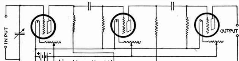
Figure 3—Resistance coupling employed with grid leaks to control grid potentials
