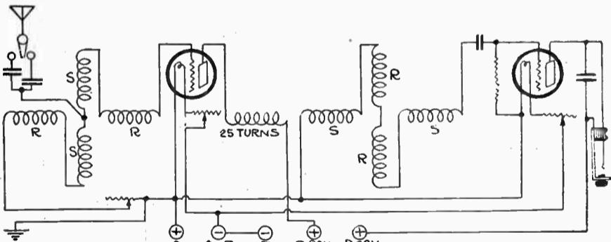
Figure 241—This hook-up was the first practical combination of regeneration and R. F. amplification.
