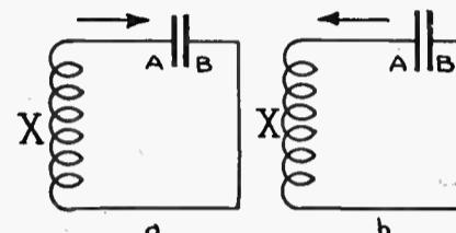
Figure 3—A diagrammatic presentation of oscillating circuit which explains condenser action
