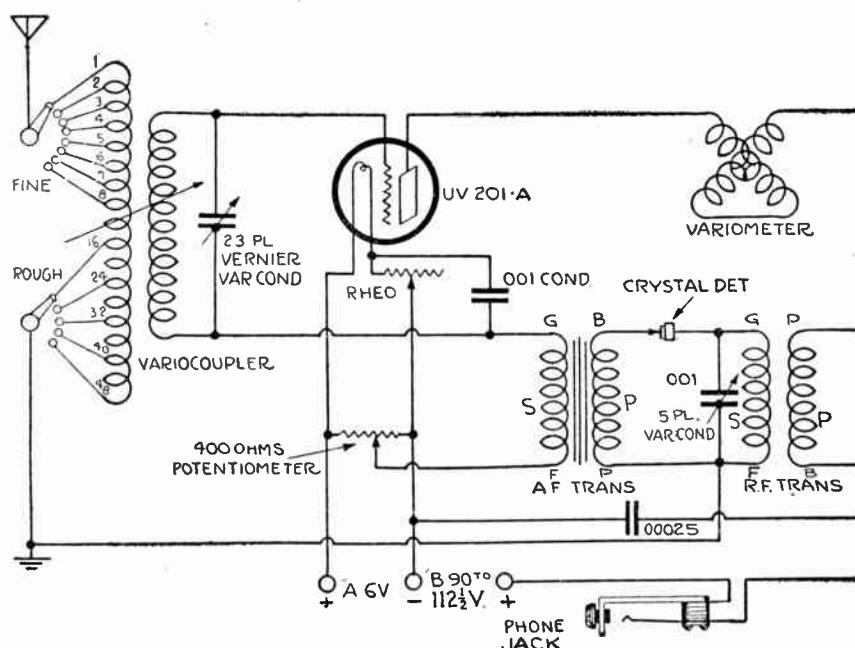
ber 20. The rotor winding is usually set in such a position that its field opposes that of the stator.
