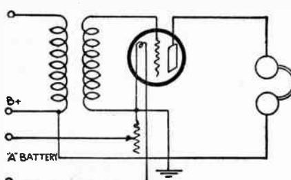
large coil. Bring the ends from the large coil out at one end and the ends from the small coil out at the other end and keep in mind which is which. The larger coil is the secondary and the smaller the primary. Wind the core with enough tape to fit well into the inside of the small coil.
