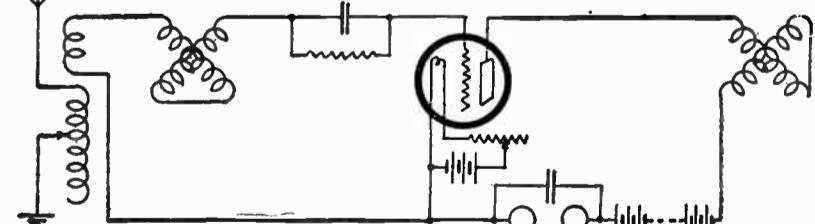
Figure 5—Three Circuit Tuner Using Tuned Plate Feed Back Switches Control Capacity Values
