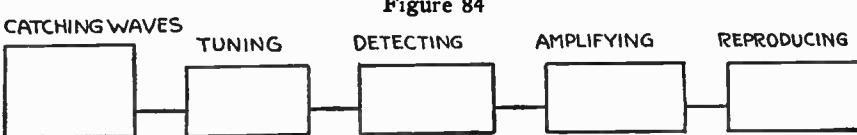
To understand a circuit it is first necessary to know what object is to be accomplished thereby. The purpose of a receiving circuit or system is to catch a portion of the transmitted wave energy and translate it back into the form of sound.
