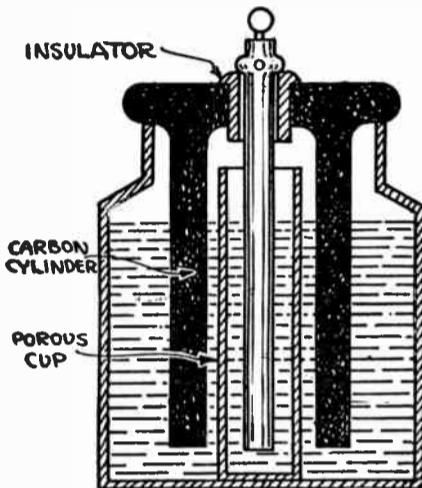
Figure 1—Cross sectional view of homemade Fuller battery for lighting tube filaments.
