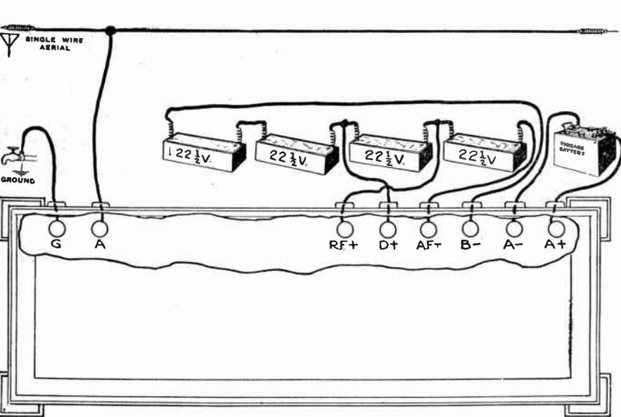
away, an outdoor aerial about sixty feet in length will usually give the best results. It should, of course, be well insulated and protected against lightning with a grounding switch or lightning arrester as specified by the fire underwriters. Even if one has an outdoor aerial at his disposal he should also provide an indoor aerial for use in receiving local stations.
