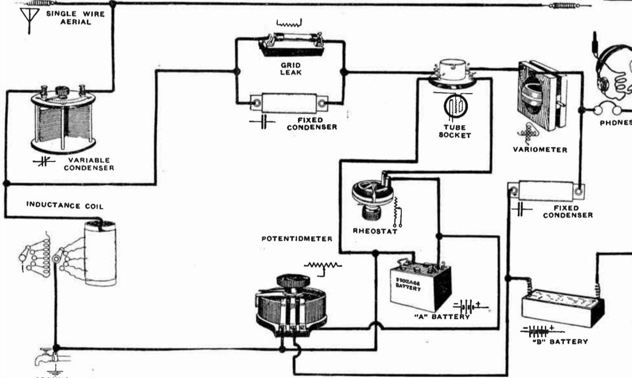
should be .002 mfd. capacity; the grid condenser .00025 mfd., and the grid leak should have a resistance of about 1 1/2 megohms. The plate circuit is controlled by means of the variometer. This variometer can be
