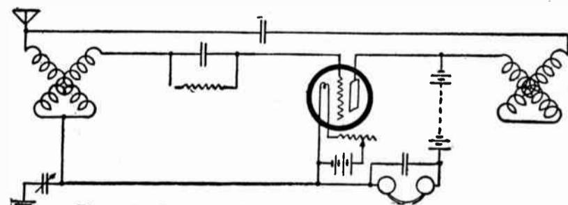
Figure 4—Capacitive Feed Back as Applied in a Circuit
