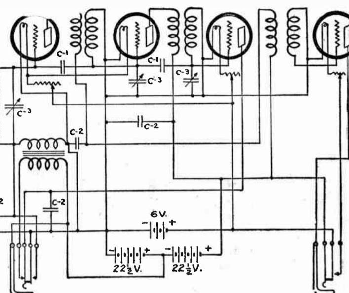
to the circuit from tube to tube which offsets or neutralizes the tube's internal capacity coupling. The values of these neutralizing capacities are so small that they are expressed in units of micro-microfarads. And one million micro-microfarads make one microfarad. Expressed in microfarads the value of the neutralizing capacity runs from .000001 to .00001 microfarad.
