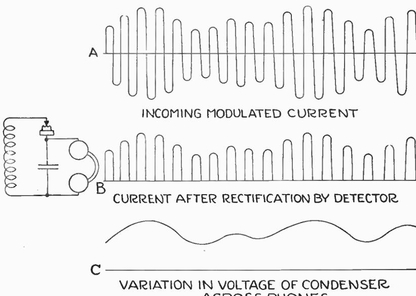
Figure 1—Showing Action of Detector in Radio Receiving Circuit
