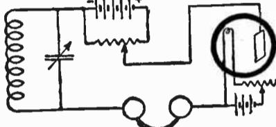
Figure 1—Fleming Valve as Used with Plate Battery
