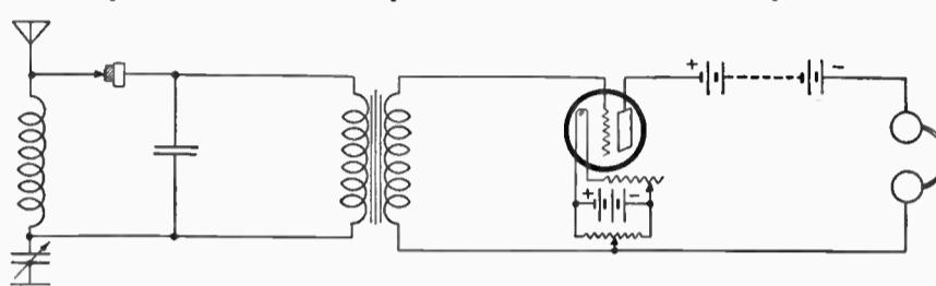
Figure 1—How a tube is used to increase strength of signals from crystal detector
