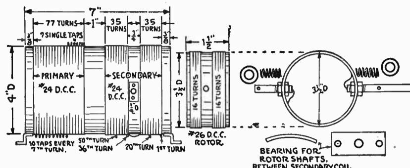
continue and wind 20 more turns, completing the secondary, which now has 70 turns of wire, or 35 turns on each side of the  $\frac{3}{4}$ -inch space, and is tapped at the first 20th, 36th, 50th and 70th turns.
