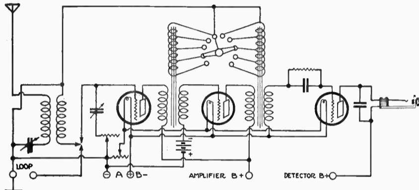
Figure 237—The "peak efficiency" of the R. F. transformers may be shifted to any frequency.
