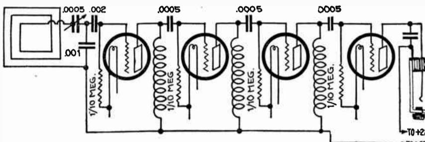
Figure 231—Three stages of untuned impedance coupled Radio frequency amplification.
