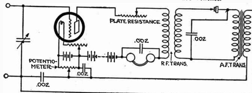
Figure 221—One-tube reflex with refinements for best operation
