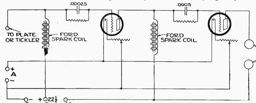
Figure 3—Two stage impedance coupled amplifier using Ford coils
