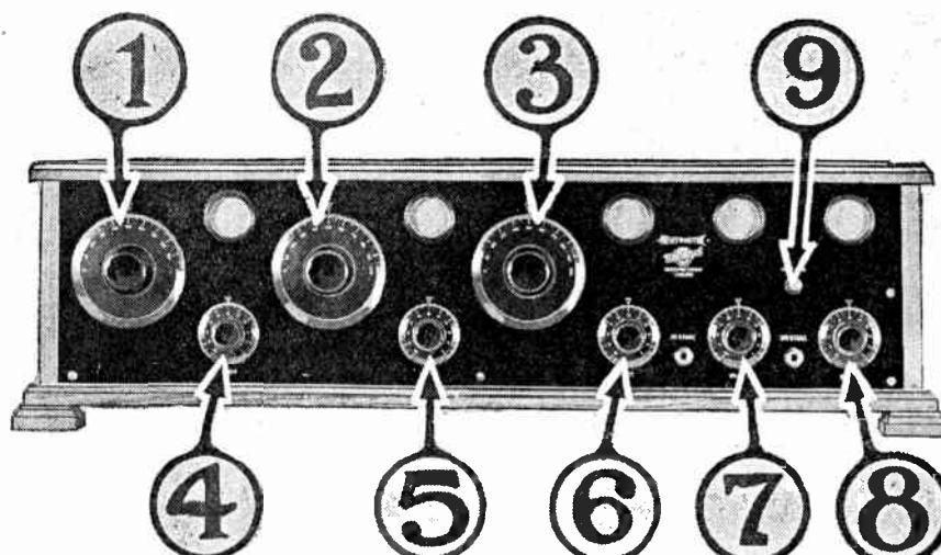
This front view of the Howard Receiver identifies each control by means of numerals. The article explains the function and operation of each one.
