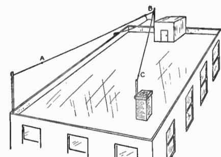
Figure 6—The arrangement of high points often makes a V-aerial possible.
