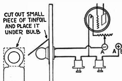
making panel lights from parts out of the junk box. A piece of tin foil, a 6-volt flashlight bulb and a socket
