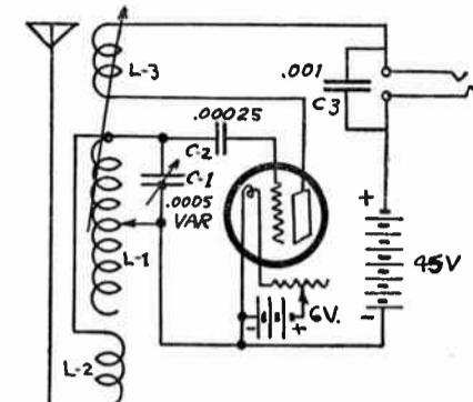
The main inductance L 1 is wound on a bakelite tube, 3 1/2 by 4 1/2 inches, using number 24 scc. wire. First tap to the grid, and then at 5, 10, 15, 30, 45 and 60 turns. A space 1/2 inch wide is left at turn 15 for the tickler shaft.
