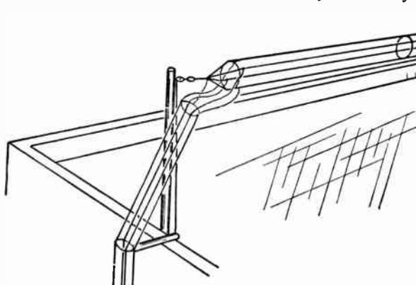
Figure 8—Cage aerial used by amateurs for transmission is good for reception
