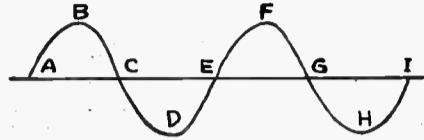
Figure 1—A diagrammatic representation of two cycles of alternating current.
