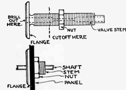
and put it in the vise with the flanged end in front. Run in a  $13/64$  or  $17/64$ -inch drill, depending on whether the shaft is  $3/16$  or  $1/4$ -inch. Drill the hole in 1 inch or more and cut the flanged end off the right length. The illustration is self-explanatory.
