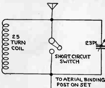
Figure 1—Series Type of Wave Trap
