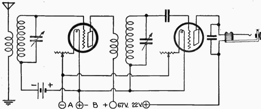
Figure 236—The fixed coupler receiver permits a stage of R. F. with but one control.
