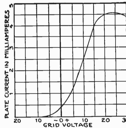
Figure 3—Characteristic Curve of Vacuum Tube Detector Showing Relation Between Changes in Grid Voltage and Current in Plate Circuit
