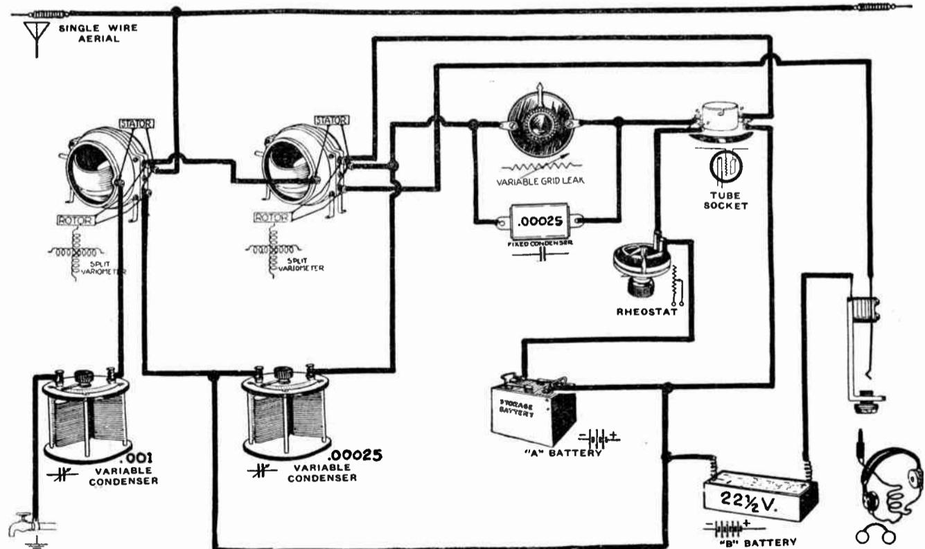
secondary circuit is tuned by means of the .00025 variable condenser. The grid leak is variable for best adjustment for various tubes. Only 22½ volts are required for the plate battery. This circuit is very selective and efficient in tuning out local Radiocasting stations. Audio frequency amplification can be added in the manner usually employed in other hook-ups.
