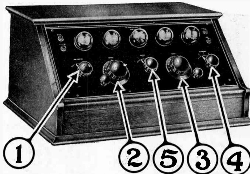
Space is provided within the cabinet for two forty-five-volt batteries or four twenty-two-volt units, and if dry cell tubes are used three additional one and one-half-volt cells can be housed inside without crowding. All binding posts are mounted on a bakelite strip inside the cabinet and to the rear of the apparatus making them convenient to get at, yet out of sight.
