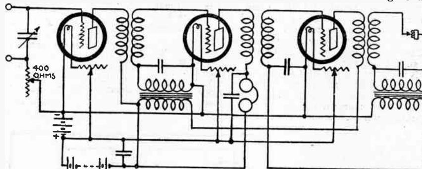
Figure 224—Inverse reflex balancing load between the tubes
