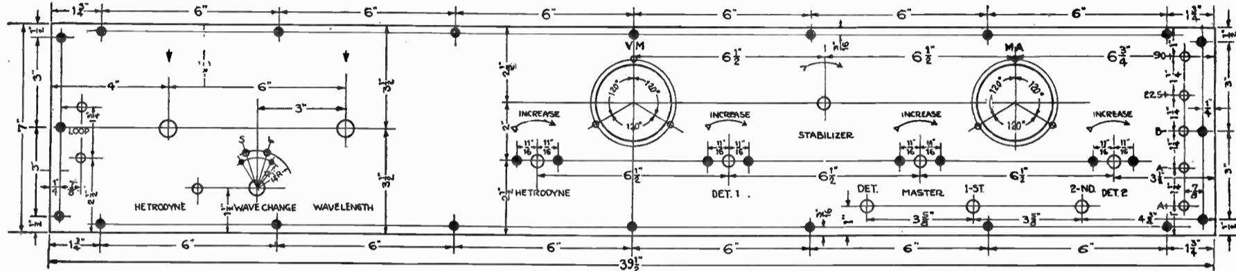
The Panel Layout for Drilling
