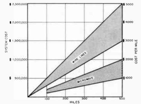
Fig. 2. The estimated initial cost of microwave and wire line installations.
