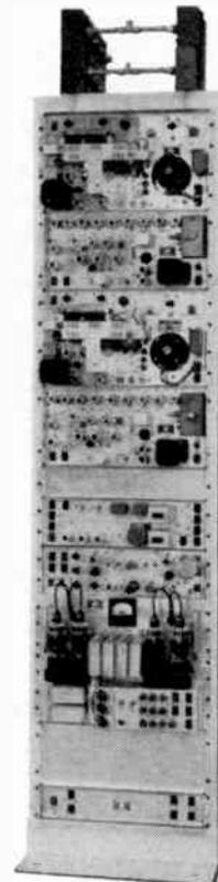
Fig. 9. Typical drop repeater station is 92 1/2" high (including filter), 21" wide, and 18" deep. Power drain is about 800 watts.
