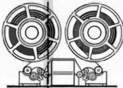
The density of recording is 200 characters per inch, permitting permanent files of data to be compressed onto a 10½-inch diameter reel holding 2,400 feet of tape. A single reel can contain over 50,000 grouped records of 100 characters each.
