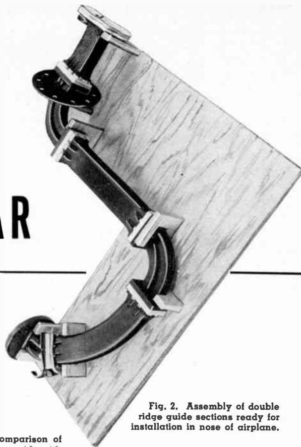
Fig. 2. Assembly of double ridge guide sections ready for installation in nose of airplane.
