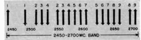
Fig. 5. Chart showing how up to nine parallel duplex systems can be fitted into the 2450-2700 mc. band in a given locality. More can be utilized when they intersect from various angles.
