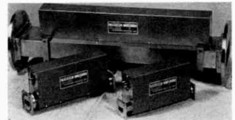
priate section of rectangular wave guide. When the discharge tube is off, the insertion loss is essentially that of the wave guide. When the discharge tube is switched on, the attenuation may be varied from less than 1 db to greater than 40 db.
