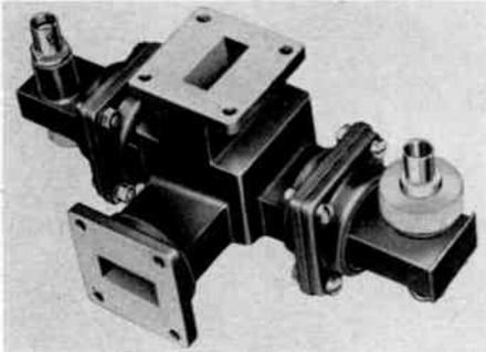
figure over its entire 12% bandwidth. In the 1" x 1/2" O.D. wave guide size, it is assembled from one precision-cast magic tee and two crystal holders.
