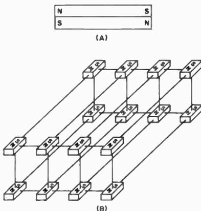
Fig. 2. (A) Each domain is completely magnetized in such a way as to produce no external field. (B) Domain structure found in silicon iron.
