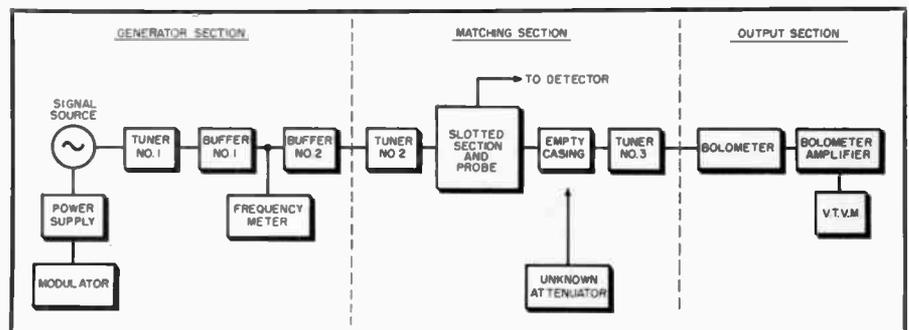
With the unknown attenuator replaced by an empty casing or line length, the output meter indication is adjusted for a convenient level  $N_1$ . Without disturbing the whole system, the unknown is inserted in place of the empty section, and the output read as  $N_2$ .  $N_1$  is then checked. If it has remained stable, the attenuation will correspond to  $\frac{1}{2}(N_1 - N_2)$  provided that the meter is calibrated for linear detection. The maximum attenuation range is approximately 50 db.
