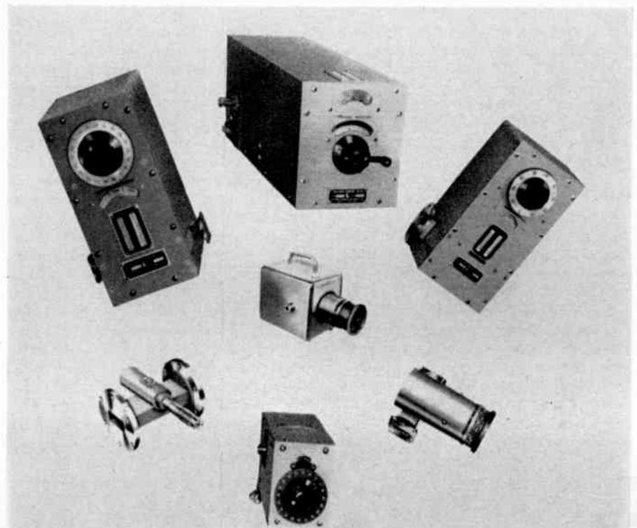
They can be operated either wide-band or selective. Selective operation is most sensitive and allows the exclusion of noise interference. The amplifier output meter scale is calibrated to read directly in VSWR when the amplifier is fed by a square-law detector such as a crystal diode.
