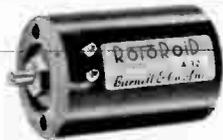
**ROTOROIDS®** A continuously variable, stepless toroidal inductor, hermetically sealed, which can provide a 4:1 range of maximum to minimum inductance in 180° rotation of a shaft.
