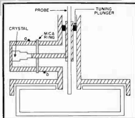
Fig. 2. Standing-wave crystal detector.
