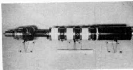
design, this new high-power u.h.f. amplifier klystron features resonant cavities completed outside the vacuum system, which is free of r.f. circuitry, permitting easy wide-range tuning and uncomplicated input and output coupling adjustment. Further information may be obtained from the Technical Services Department of *Eitel-McCullough, Inc.*, San Bruno, Calif.
