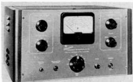
db. This amplifier is well suited for use with slotted sections in measuring VSWR over the wide range of 1.0 to more than 100. With a 15-cps bandwidth, the noise level is only 0.03  $\mu$ v.
