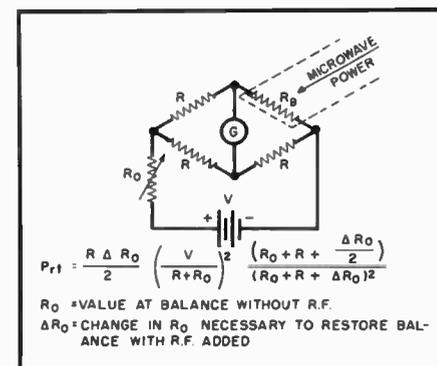
Fig. 10. Wheatstone bridge circuit for measuring microwave power in a bolometer.
