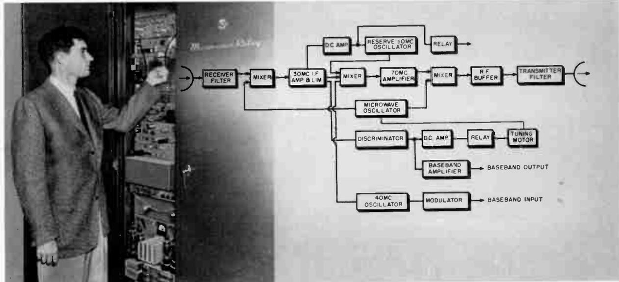
Fig. 1. View of the over-all equipment (left) and a block diagram of a typical branch through a repeater station. Stages shown are in the transmitter and receiver units.
