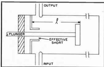
Fig. 7. Cross-sectional view of a TE<sub>011</sub> mode cavity resonator frequency meter.
