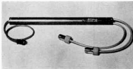
*ries, Inc.*, 711 Hamilton Ave., Menlo Park, Calif., the unit requires a 400-gauss field and a 1200-volt regulated power supply. Approximate operating characteristics are 30-db gain and 5-mw. output.
