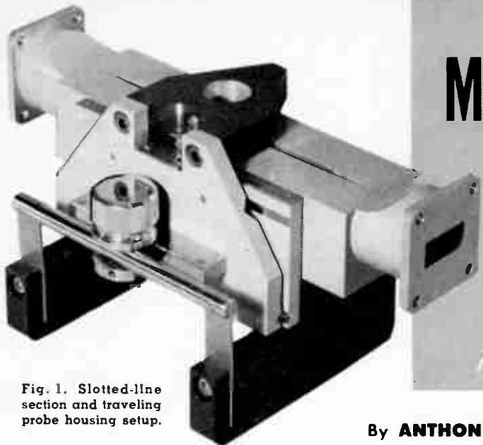
Fig. 1. Slotted-line section and traveling probe housing setup.
