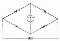
Fig. 5—Strain gauge is a Wheatstone bridge.
