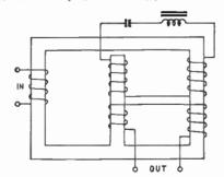
The output voltage is due mainly to the winding around the right-hand leg. This is opposed and stabilized by the voltage induced in the leg winding which is more sensitive to center load changes. A third winding is connected to a series condensor and iron-core inductance which resonate at the third harmonic of the line fre-quency. The harmonic is greatly reduced, leaving a pure output wave.
