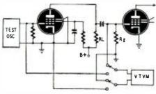
Fig. 3-V.t.v.m. measures shunt capacitance.
