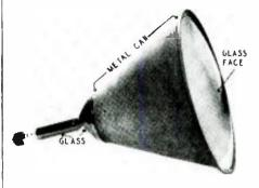
is used for the face. Advantages include: lighter weight (the new tube weighs only about one-sixth as much as a 15-inch all-glass tube); larger viewing area (144 square inches, compared with 115 for a standard 15-inch glass tube); and better shielding from ambient light.
