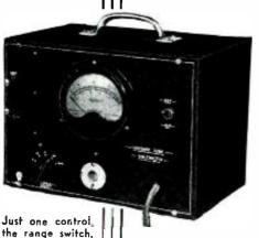
A practical instrument which uses an extra amplifier tube for the lower-voltage ranges
