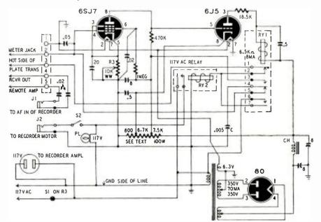
Fig. 1—Receiver develops voltage to cut off 65J7 and trigger relay in plate circuit of 6J5.
