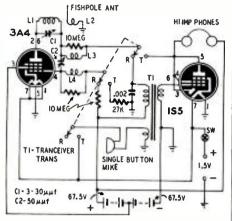
are paralleled for 1.5-volt operation. The 1S5 is modulator and audio tube.
