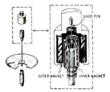
Fig. 2—The shaft is suspended by magnets.
