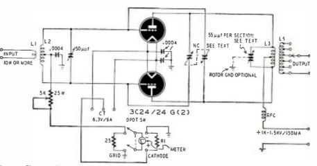
Fig. 1-This simple push-pull amplifier can be built on the TU-10-B chassis in a few hours.
