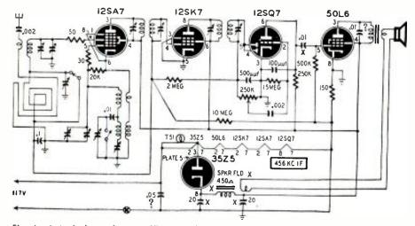
Fig. I—A typical a.c.-d.c. set. X's mark the common sources of hum; 7's occasional ones.
