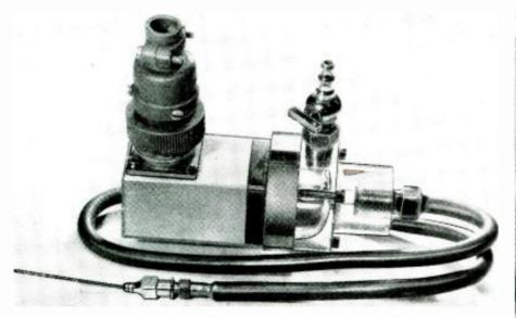
Photograph of the blood-pressure measuring device diagrammed in Fig. 2. Plug is for wires. NOVEMBER, 1948
