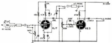
Fig. I-A simple but efficient visual signal tracer. The 6E5 is detector and indicator.
