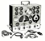
Output is controlled by a shielded attenuator. To compensate for the loss in gain usually present at the higher frequencies, output of all generators in-creases about five times at the high frequencies over that at the low end of
