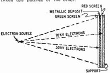
In the presence of 50 kv electrons the green screen becomes dark after developing. If the entire plate is then held to a light these areas will look red. When the plate is exposed to 70 ky electrons, the red screen becomes dark. Therefore the plate looks green when held to a light. Different color shadings correspond to slightly different electron velocities.
