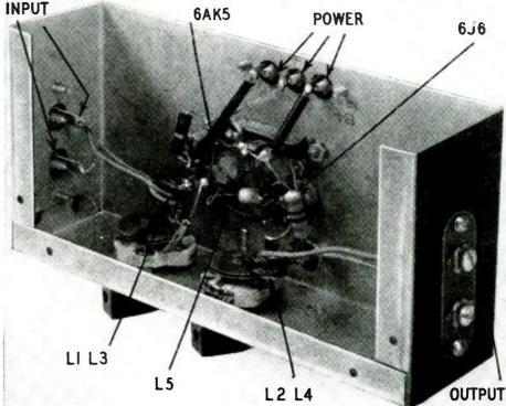
Fig. I—Unit is a cascode with double tuning. Underchassis view. Parts layout and manner of winding coils can be seen from the photograph. RADIO-ELECTRONICS for
