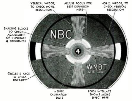
Fig. I—This typical test pattern helps owner and serviceman adjust set for best picture.
