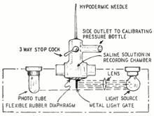
Fig. 2-Taking blood pressure with phototube.
