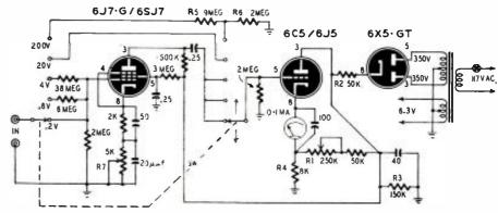
Fig. 1—Pin numbers of detector tube refer to 6J7-G only. R1 is the zero-adjustment control. RADIO-ELECTRONICS for
