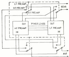
Fig. 2-Proposed low-high switching circuit.
