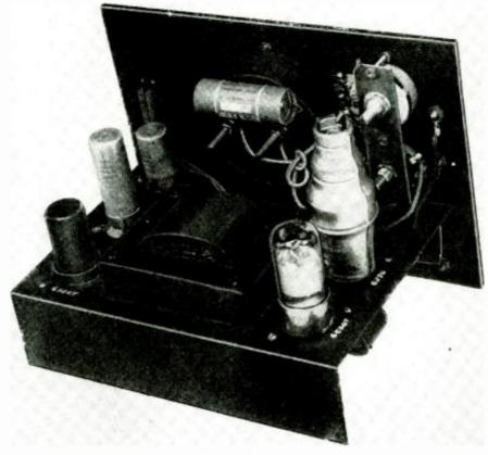
The chassis layout. Notice the shield covering the 6J7-G. RI and R7 are on strip at right.
