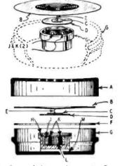
Fig. 2-Parts of the earphones. A--Cap made of plastic: B—Diaphragm; C—Reinforcing disc on armature; D—Armature; E—Wire connecting armature to diaphragm; F-Cushion ring; G-Plastic case; H-Brass shell; J-Coil winding; -Alnico magnet. Units receive and transmit.
