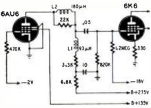
Fig. 8-Commercial series-shunt high peaker.
