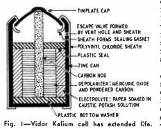
cules to form water. Short-term polarization thus occurs because of the formation of a film of hydrogen gas round the carbon rod. The internal resistance goes up, and down goes the e.m.f.
