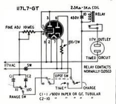
components. The maximum time can be increased somewhat by adding a third position to the range switch, with a 20to 40-µf paper capacitor.
