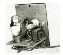
The panel shelf makes construction easier. RADIO-ELECTRONICS for
