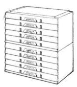
CAN BE STACKED ON EACH OTHER A dovetail joint is provided on top and bottom of each cabinet so they can be stacked
