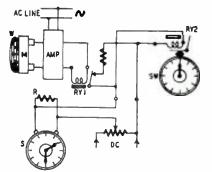
watch then stops and indicates the speed of the test watch. If W runs correctly, this happens exactly 30 seconds later. If it is too slow, it occurs later, and if two fast, the beats coincide earlier. The stop watch indicator travels around once every 30 seconds, and its face is calibrated in seconds per day to show the speed of the watch. W.
