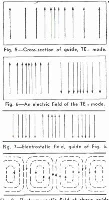
Fig. 8-Electromagnetic field of above guide.
