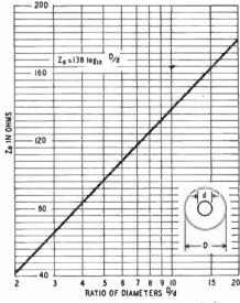
Fig. 5—Impedance chart for concentric lines.
