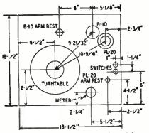
Fig. 4—The drawing shows motorboard layout.
