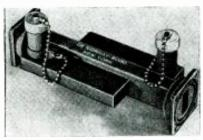
Fig. 15—Example of a bidirectional coupler.
