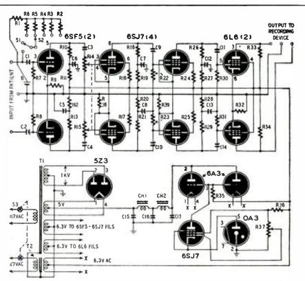
Note-screen resistor of 6SJ7's should be connected to junction of tubes plate resistor, decoupling capacitor, and decoupling resistor instead of direct to the B-supply.
