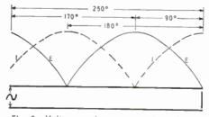
Fig. 3-Voltage and current on shorted line.
