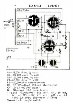
is used as a simple diode rectifier for the negative reference voltage. Two type NE12 neon lamps serve as the voltage standard, and one of these also acts as a pilot light, visible at the front of the chassis.
