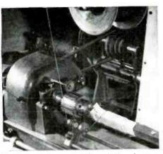
Should an end turn cut through the glassine, lay a strip of paper under it as shown above,
