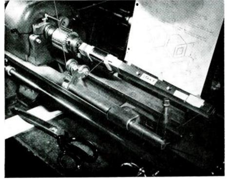
Above, left—First layer wound in place. To start second layer insert glassine paper under wire so that wire is at least one-eighth inch from paper's edge, and roll it on with the next turn of wire. (Photo right.) Paper secures and stiffens ends of windings.
