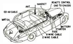
Fig. 2-Installation of components and leads.
