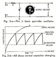
age of V. When the capacitor has charged enough so that its voltage equals the tube breakdown value, the gas within the tube ionizes. The tube conducts.
