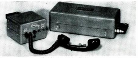
Raytheon transmitter-receiver (right) and control box (left) show compactness of equipment.
