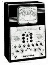
tubes. A 9-inch illuminated scale reads REPLACE, DOUBTFUL, and GOOD. The tester uses the dynamic mutual conductance circuit, and the meter shows ranges of 3,000, 6,000, and 15,000 micromhos as well as the zone markings mentioned
