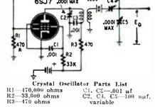
mitter or as a crystal test set. Frequency and amplitude stability are excellent. In addition, the frequency is variable over a limited range. Feed, back is adjustable to accommodate different types of crystals.
