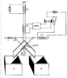
The pivoted gate is fixed to a lever L at right angles to it. Normally L is forced to the left by a spring S. This position is shown by full lines in the frawing. When L is forced towards the solenoid S3, the lever and gate take the position shown by dotted lines. Note that in the first case only the passage leading to A, in the second case only that to B, is open.
