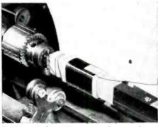
Finishing winding. Place paper loop as shown, wind a few turns over it, pull up loop ends and continue. On next (last) layer pull end
