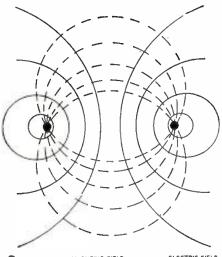
WIRE ------------------------------ELECTRIC FIELD Fig. I-End view of line and fields around it.
