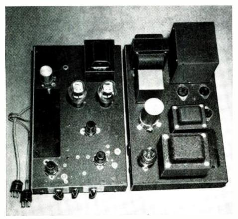
Fig. 5-Use of separate chassis for amplifierand power supply helps to reduce hum pickup.
