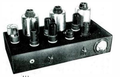
Front view of the phase-modulated exciter. The signal of a low-frequency crystal is multiplied eight times to hit 80 meters.
