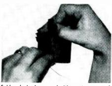
Soldered wire is covered with another piece of insulation, held down with some coil cement.
