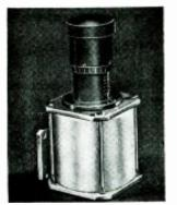
Fig. 13—Cavity wavemeter for 8400-9800 mc.
