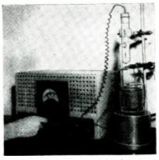
The regulated supply in use for electrolysis.
