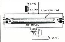
high-voltage a.c. This ionizes the gas sufficiently to allow the 117-volt line current to keep the tube lit. After the lamp is started, the coil can be removed. DONALD G. BERLYER, Ballarat, Australia
