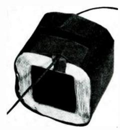
Adhesive strips make external connections stronger. Whole winding may be taped also.
