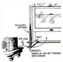
The antenna is a 10-foot collapsible rod type, obtained from surplus. It is mounted on a strip of wood. The other end of the strip is bolted to the window sill.
