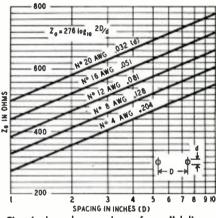
Fig. 4-Impedance values of parallel lines.
