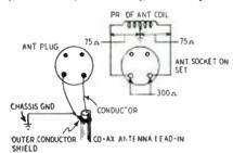
quality will be improved if the unused part of the coil is shorted out by grounding the remaining terminal. This connection can be made on the antenna plug by connecting the co-ax across the 300-ohm terminals and grounding the outer conductor to the chassis as shown in the drawings.
