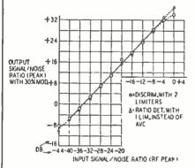
Fig. 7-b—Limiter helps ratio detector.
