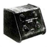
Dual tuning controls are provided for separate adjustment of sound and picture signals. The dual tuning is said to improve the over-all selectivity so that much interference is minimized or eliminated. Another cantrol varies the booster's gain so that the receiver is not overlaaded by strong signals. The on-off switch controls the internal power supply and also removes the booster from the antenna circuit.
