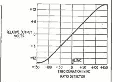
Figs. 6-a, 6-b—Curves of phase discriminator and ratio detector, no noise.
