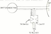
Fig. 5-TR switch in antenna circuit.
