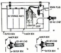
Fig. 2—Details of noise generator.
