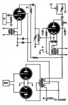
The modulation transformer has two secondaries. One modulates the exciter screen; the other modulates the plates. The audio voltages applied to the exciter elements should be propor-tional to their d.c. potentials for lowest distortion.
