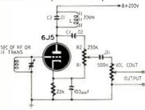
from a bridge composed of the internal resistance of the tube. C1. R1, and R2. At frequencies above and below the resonant frequency of L-C2, the plate-circuit impedance is low and most of the audio voltage is developed in the cathode circuit. If R1 and R2 are equal and the reactance of C1 is low, the output voltage will be half that developed in the cathode circuit. If the impedance
