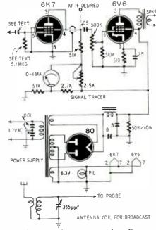
Fig. 2—Complete construction diagram.
