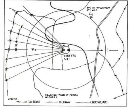
Fig. 2—Intensity readings were taken at 9-degree intervals around antenna.
