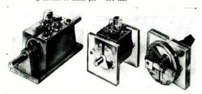
ture transmission. The Institute's Department of Electrical Engineering has developed three new u.h.f.-to-v.h.f. converters which are both simple and inexpensive. With such a converter, a standard receiver will need no internal modifications to receive u.h.f. programs.
