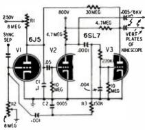
blocked and discharges abruptly when the tube conducts. The sawtooth voltage is amplified by V2 and applied to one of the kinescope deflection
