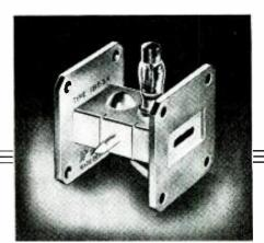
Courtesy Sylvania Electric Products Inc. A TR assembly for waveguide insertion
