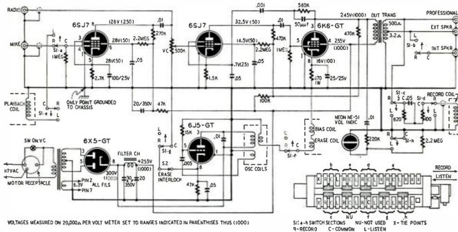
Complete amplifier schematic. Apparently the single-point ground is largely responsible for the complete absence of hum.
