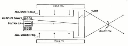
A partial cross section of the image orthicon, showing path of the electrons.
