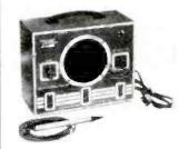
frequency probe is provided. The instru-ment is isolated from the power line by a transformer.
