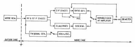
Fig. 1—Equipment used to compare ratio detector with limiter-discriminator.
