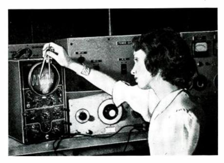
Machinist's dividers are used to compare shutter opening with audio sine waves.
