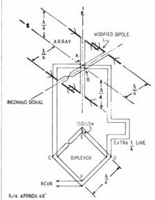
Fig. 2-Antenna array with diplexer.
