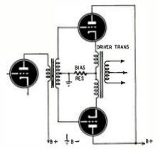
Fig. 3-A cathode-coupled driver stage.
