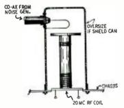
Fig. 3-Method of injecting the noise.
