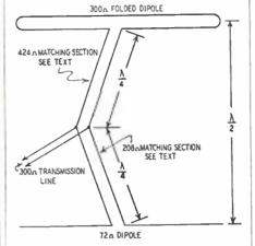
The electrical length of the quarterwave section can be calculated from
