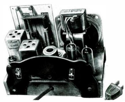
Rear view of the permeability-tuned receiver. Tuner is in upper left corner.
