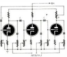
Each stage has an R-C phase shifting network. If each stage is designed to shift the voltage by 120 degrees, the total is 360 degrees. Since the output of the last stage is in phase with the input to the first, and is fed back to it, oscillation takes place.
