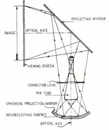
Fig. 4—A typical TV projection system.
