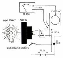
Fig. 4—A setup for synchronizer tests.
