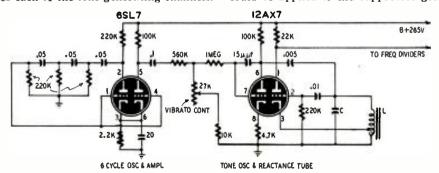
The low-frequency oscillator and a single tone-generating oscillator and reactance tube are shown in the diagram.
