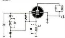
coil L1 is added to accentuate the higherorder harmonics. With the usual capacitor alone these higher frequencies are bypassed to cathode and lost. A second coil L2 is added in the cathode circuit instead of a bias resistor. Here again the harmonics are strengthened.
