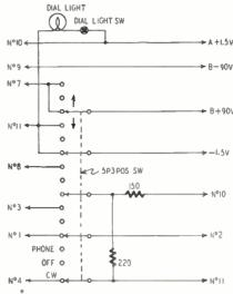
NOTE - NUMBERED LEADS GO TO TERMINAL ON STRIP ON RIGHT SIDE OF CHASSIS
