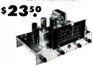
Ideal AC operated superheterodyne receiver for home use or replacement in console cabinet. Comes complete with attractive metal panel for cabinet mounting. Modern circuit uses 12K8 converter, 12SH7 input IF stage, 12C8 output IF stage and first audio 12A6 beam power output stage, 5Y3 rectifier. Excellent sensitivity for distant reception with selectivity which effectively separates adjacent stations.
