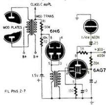
class-C plate voltage below zero on peaks. If the indicator is allowed to protrude from the panel of the indicator, it will be visible over a wide angle and some distance away—a feature not possible with other types of indicators.
