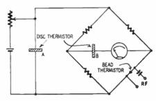
Unfortunately the head is affected by changes in ambient temperature as well as current flow. For example, if there is a drop in room temperature, the resistance of the bead drops. In this circuit two disc thermistors are added to correct the error. The disc type is affected chiefly by ambient temperature rather than current flow.
