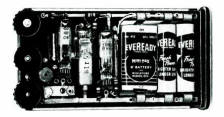
This side of chassis shows now the tube "pins" are bent and pushed in sockets,
