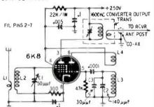
Coils are wound with No. 22 enameled wire on 11/4-inch plug-in forms. The number of turns per winding is shown in the table.
