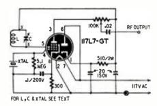
tal they are designed to work with. The 1.25-mh inductor may be half of a 2.5-mh r.f. choke.—Harry C. Aichner, Jr.
