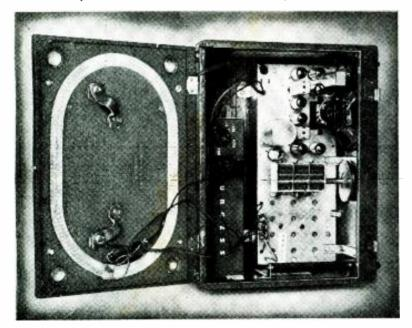
A single pack supplies A- and B-power. A broadcast loop is inside back cover-
