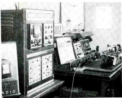
This is the service-bench section of Ward Custombuilt Radio in New York City. The test cabinet has four panels of instruments and is mounted on a roll table so that it can be used where needed. All tables and racks are made of steel. Fuses are provided for all bench a.c. outlets and a master switch turns off all power. An adjustable fluorescent lamp over the bench illuminates the critical spots.
