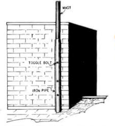
A 10-meter beam, on a 15-foot mast, supported in this way, stayed up through-out the winter without guying.
