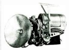
Scanner unit of the Ekco cloud and collision warning radar. This is 3-cm system designed to warn aircraft pilots of storm clouds and other aircraft as far away as 40 miles. The entire radar setup consists of seven separate units, E. K. Cole, Ltd., manufactures the system.
