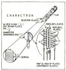
Fig. 1—Construction of the Charactron.
