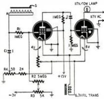
tiny flashes. Also, charged sheets are difficult to handle because they tend to adhere to nearby nonconductors. This simple discharger includes an indicator to show when correct discharge is
