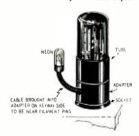
Fig. 1—A tube in the adapter assembly.
