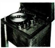
The recording or playback time of this magnetic recorder is 80 minutes. It employs a 1,000-yard-long plastic tape.
