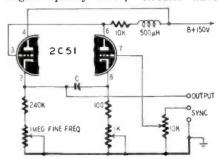
been developed, but they are seldom used in low-cost equipment because they require several tubes. A new widerange sweep generator having a range from 15 cycles to 500 kc was described in The Review of Scientific Instruments. The circuit is shown here.
