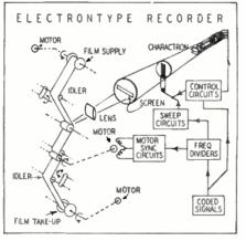
Fig. 2—Complete Electrontype recorder.
