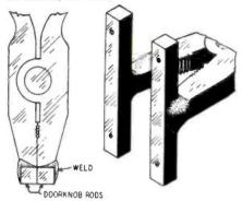
Take two pieces of doorknob rods and weld them to the jaws of a pair of lineman's pliers as shown in the drawing.
