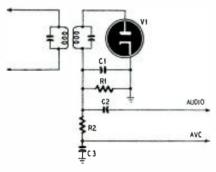
Fig. 1—The sources of a.f. and a.v.c.
