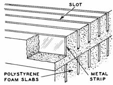
Fig. 4—Cross section of magnetic lens.
