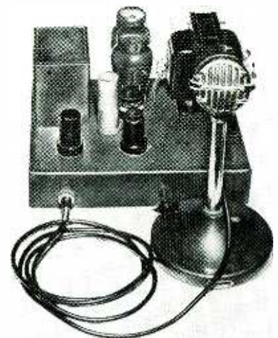
An audio amplifier having two voltage amplifier stages and push-pull output.
