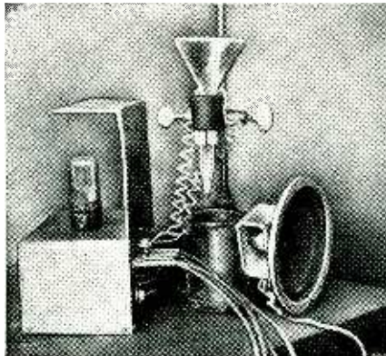
Fig. 2—The complete rain indicator. Sensitivity depends on the funnel size.
