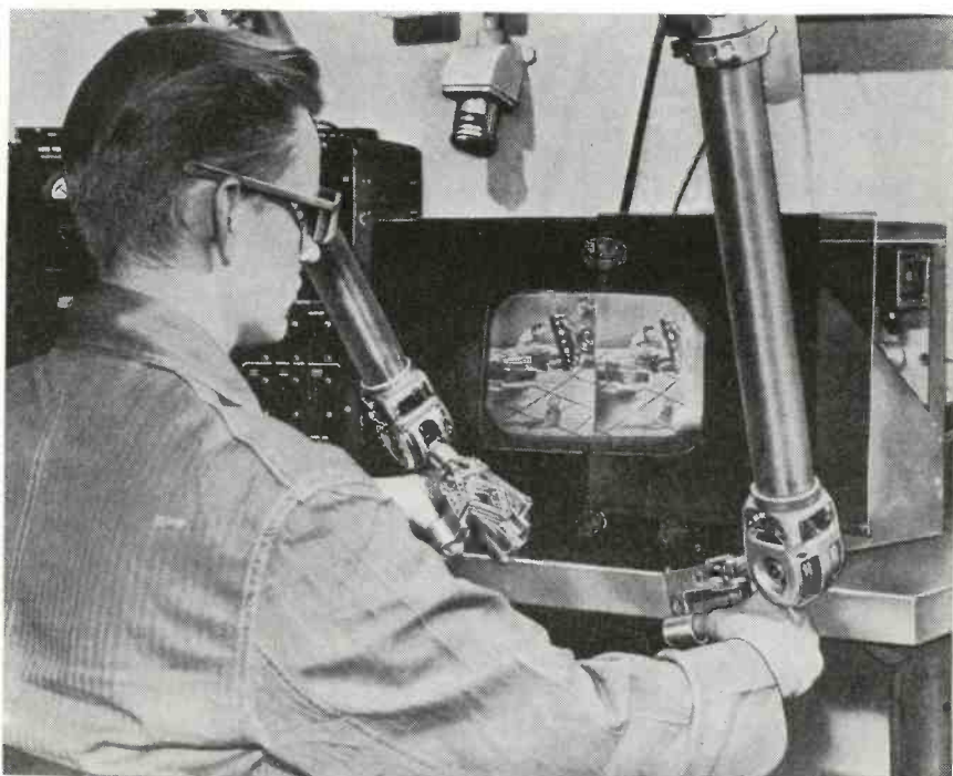
Carl A. Hermanson of the Argonne National Laboratory performs remote control operations which he observes with Du Mont three-dimensional stereotelevision.
