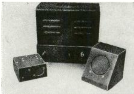
The sound alarm's three components are shown in this photo. The alarm device is at left, the amplifier center, and the speaker used as a pickup is at right.
