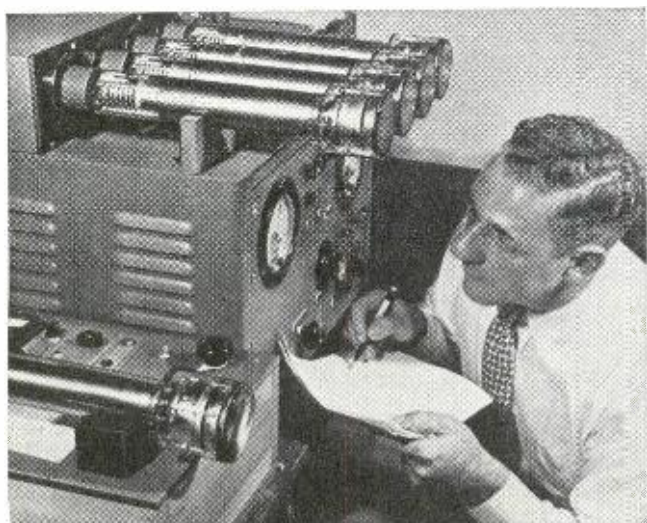
Here, in a testing battery at RCA Tube Plant in Lancaster, Pa., RCA image orthicon pick-up tubes get the final seal of approval from an engineer.
