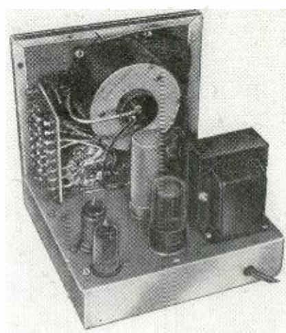
Rear view photo of the meter showing the parts layout. The voltage dividers are on the mounting boards at the left.
