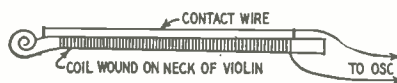
Fig. 3—One tone generator has the variable oscillator coil wound on a violin neck. The pitch is varied when the contact wire above this coil is pressed.
