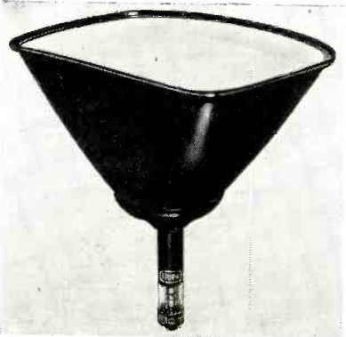
Electrostatic focusing is used in the RCA 17GP4, a 16 kv metal-shell type tube.
