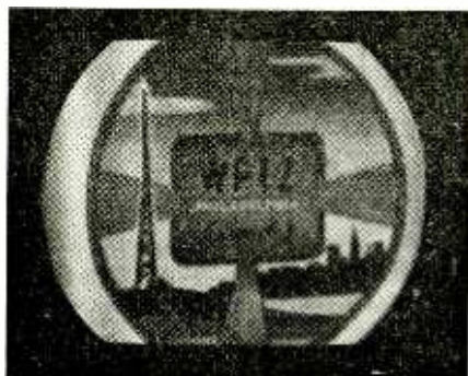
Fig. 1—"Blooming" is caused by low second anode voltage. Note poor detail here.
