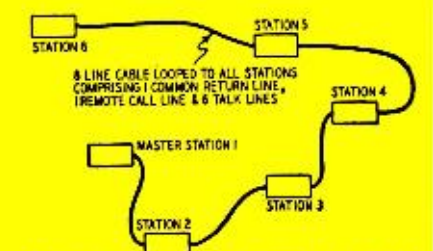
Fig. 7—Loop wiring method is the easiest and most economical way to connect intercom system elements.
