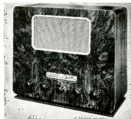
Fig. 4—AM/FM receiver designed for tests is linear, \pm 2 db, 30-12,000 c.p.s.
