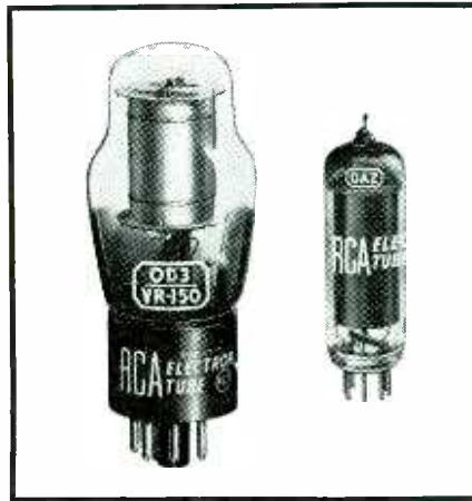
Fig. 1—Cold-cathode gas tube OD3. The small tube beside it is an OA2.
