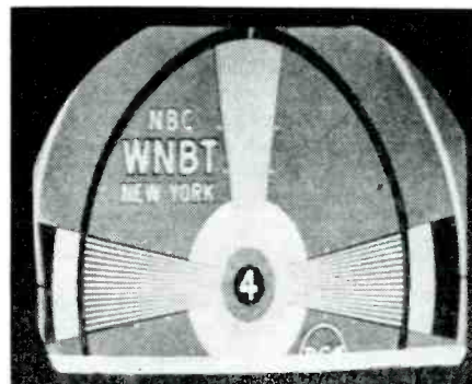
Fig. 2—What a leaky capacitor can do.
