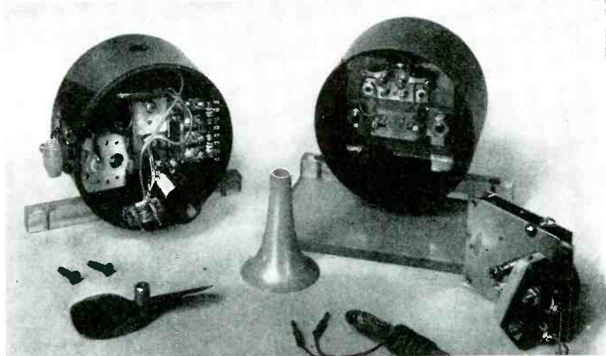
Receiver (left) and motor (right) with reducing gears, horn and other equipment. Courtesy Scientific Products of Indianapolis
