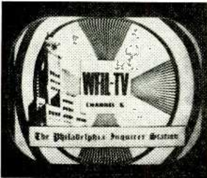
Fig. 3—Bending at top of the picture is the result of insufficient sync pulse and trouble in the sweep circuit.
