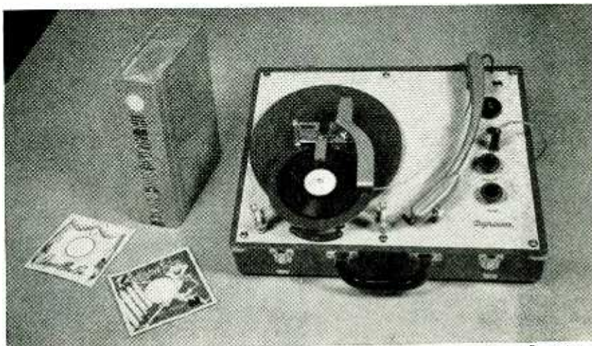
Photo of a 16-r.p.m. record and adapter on a standard Dynavox record player.
