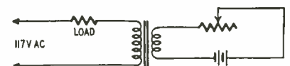
Fig. 2—Basic magnetic amplifier circuit. The magnetizing effect of the d.c. controls the permeability of the iron core.
