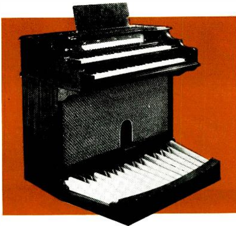
Fig. 1—The Model J Minshall Electronic Organ has two manuals, pedal clavier, and built-in amplifier and speaker. Other models have external tone cabinets rated at 20 and 40 watts. The instrument is all-electronic, with tube generators; tones are colored by formant method.
