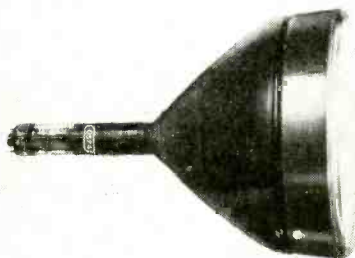
The 10SP4 is a 10-inch monitor tube.
