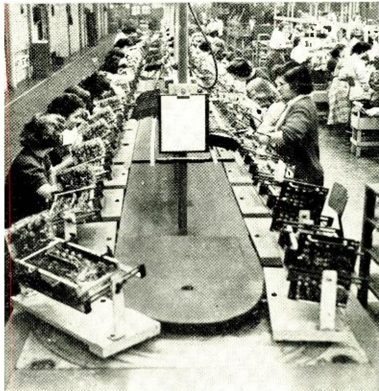
U.S. jet-fighter guns find targets automatically with these small radar units. Highly successful in Korea, and mass-produced on these high-speed General Electric assembly lines, they are now standard equipment for all U.S. air arms.
