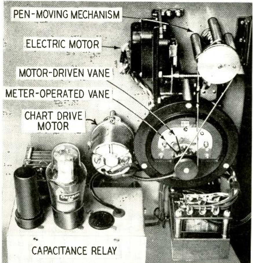
Photographs courtesy Wireless World A Servograph assembly. Action is reversed by merely uncrossing the vane drive belt.
