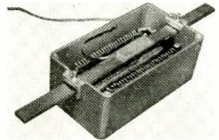
Fig. 8—Inside the expression control. Sliding bar contacts fixed resistors. Attenuates volume in 60 small steps.
