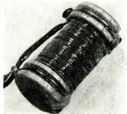
Photo B—Construction of pickup coil.
