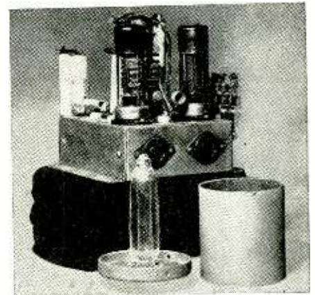
The speaker unit with its r.f. exciter.
