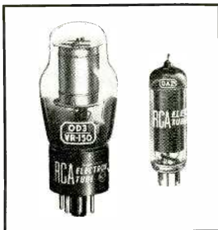
Fig. 1—Cold-cathode gas tube OD3. The small tube beside it is an 0A2.
