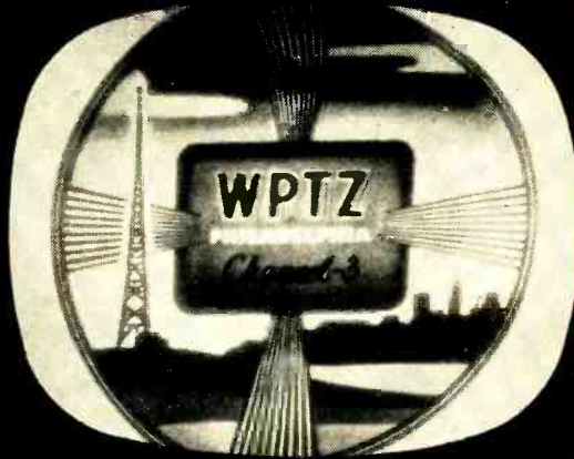
Fig. 1—Bending of vertical picture lines may have several causes. See text.
