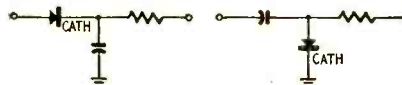
Fig. 2—Series (left) and shunt detectors. The series resistors prevent the scope input capacitance from shunting the detector and reducing the output.
