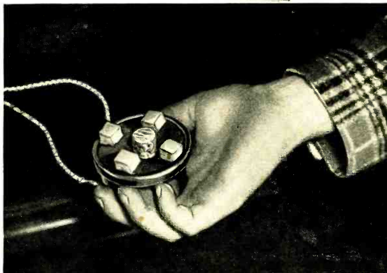
Fig. 2—The completed contact microphone, with four rubber support blocks mounted on the face of the earpiece cover.
