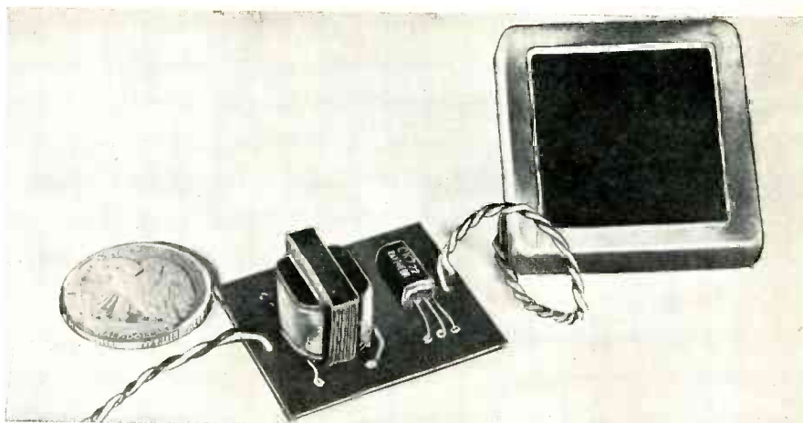
Oscillator is little larger than half dollar. Photocell power supply is at right.
