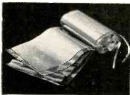
Unrolled view (one-third size) of capacitor unit wound with "Mylar." The transparent film is only 0.0005" thick yet stands handling without breaking.
