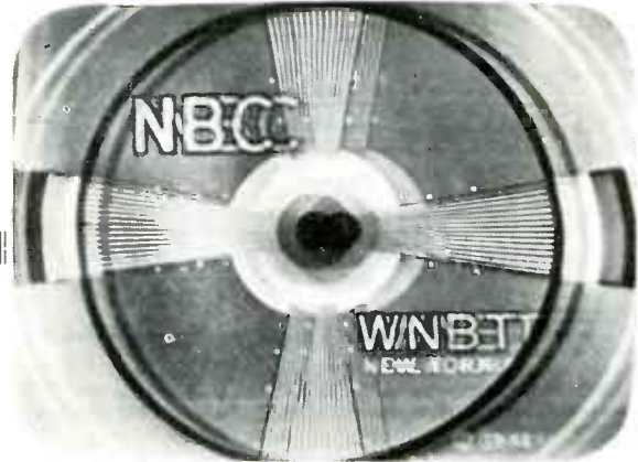
An example of the type of intermittent horizontal picture displacement discussed in one of this month's clinic questions.
