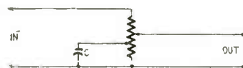
Fig. 1—Compensated volume control. As the slider moves down to reduce volume, capacitor C bypasses high frequencies around the lower resistance element. This introduces an apparent increase in low-frequency response.
