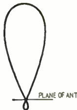
Fig. 5—Directivity pattern of the end-fire arrangement shown in Fig. 4.
