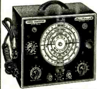
• Tubes used: 1-6BE6 as R. F. Oscillator, mixer and amplifier. 1-6BE6 as Audio Oscillator. 1-6HG as Power Rectifier.
