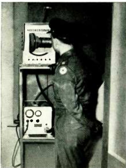
Capt. Guy F. Bohn, bomb-renovation officer, watches plug-unthreading process on the television screen inside the bombproof shelter where he controls the entire dismantling operation as he watches the screen for any sign of untoward activity during the process.
