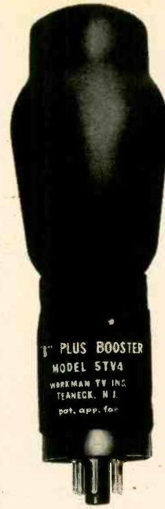
Left—Workman-TV 5TV4 "B plus Booster" replaces 5U4 where line voltage is low. Below—New Tung-Sol 6AU4-GT damper diode is designed for 90° deflection systems.
