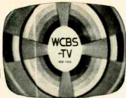
Fig. 3—White vertical bar and compressed center caused by overdrive.
