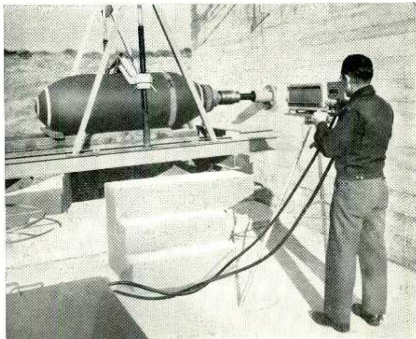
Capt. Guy F. Bohn, bomb-renovation officer, watches plug-unthreading process on the television screen inside the bombproof shelter where he controls the entire dismantling operation as he watches the screen for any sign of untoward activity during the process.
