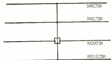
Fig. 1—Basic Yagi antenna. Extra directors may be added to raise gain and sharpen forward-directivity pattern.
