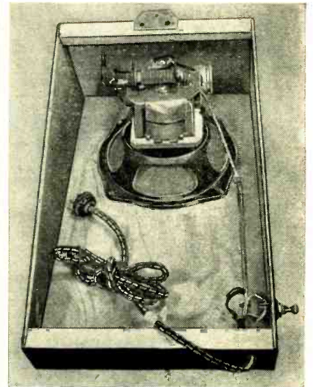
The author's remote-speaker assembly. The sloping-front wood baffle can stand by itself or hang on a wall. Mounting the speaker off-center helps to flatten out the frequency response.
