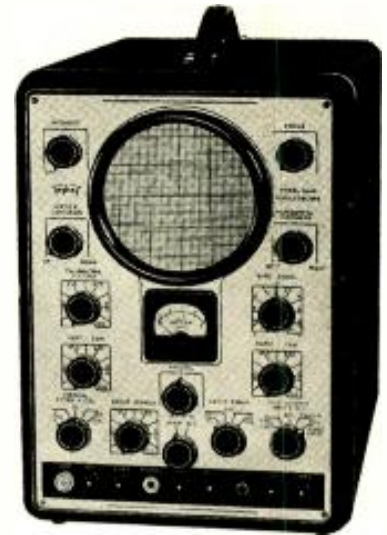
A commercial oscilloscope with built-in 10-range voltage source and meter for peak-to-peak screen-scale calibration.
