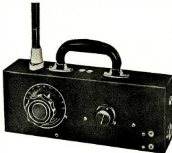
Photo A (left); Photo B (below)—Front and back views of the high-gain portable. The Vari-loopstick is mounted on the strap across the back of the tuning capacitor. The socket at the side can be used to check battery voltages, or for plugging in an external power supply.
