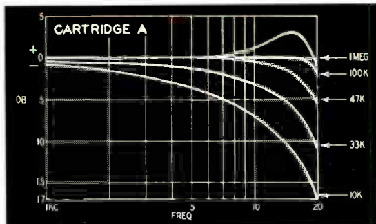
Fig. 1—Frequency response vs load of moving-coil cartridge.
