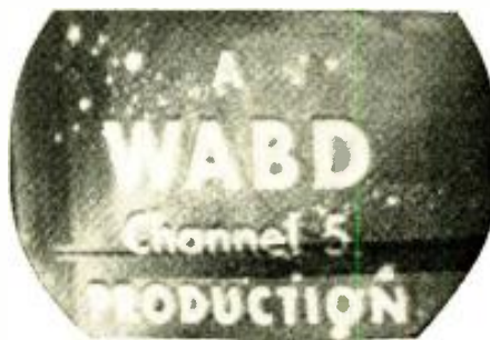
Fig. 2—Adjacent-channel video on distant channel 4 from local channel 5.
