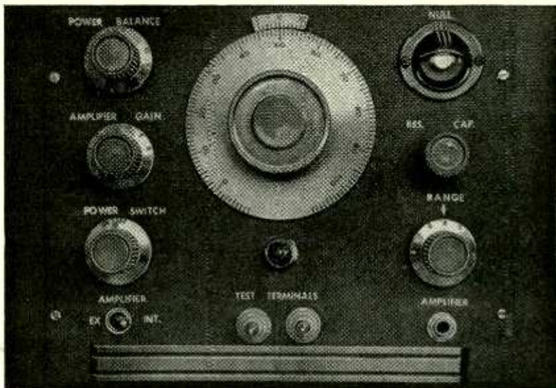
Front view of R-C test bridge. Main dial must be carefully calibrated.
