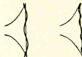
Fig. 4—Diagram shows side view of nodes in an exponential diaphragm.
