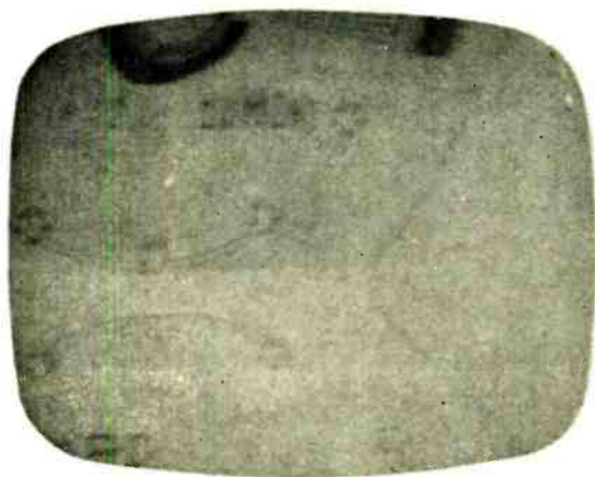
Fig. 3—Poor contrast, snow, and poor sync may result from excessive bias.
