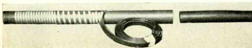
The antenna is composed of a magnetic core (right) inserted into a cylinder around which a conductor is wound.
