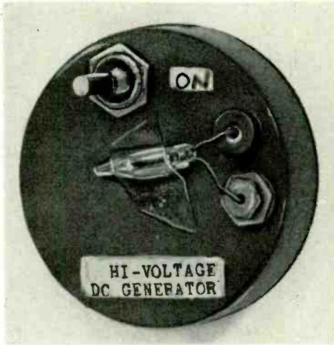
Front view—neon lamp acts as indicator.
