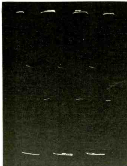
Fig. 5—Output waveform of one-shot multivibrator at 100 kc, 10 volts p-p.
