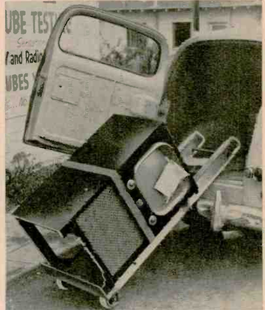
Fig. 4—Ready to load. Lift dolly to horizontal position and slide forward. Close door. Drive off.
